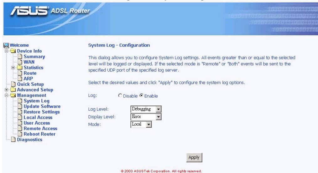
Figure 7.3 System Log Configuration
