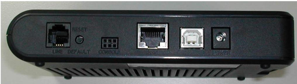
**Figure 2.3 Rear Panel Connections**
