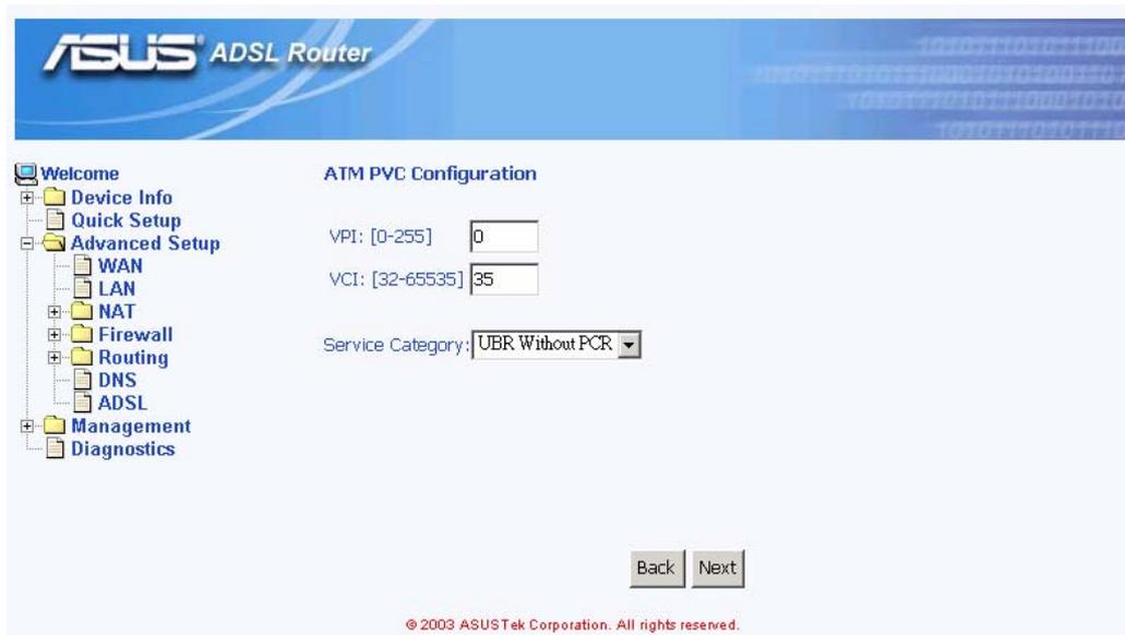
**Figure 6.2 ATM PVC Configuration**
