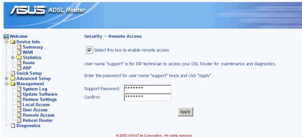
**Figure 7.8 Remote Access Setup**
