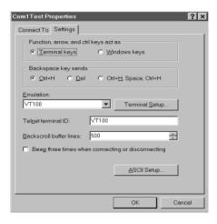
7. Change the settings (if necessary), so that they match the settings shown in the dialog box, then click **ASCII Setup...** The *ASCII Setup* dialog box comes up:
