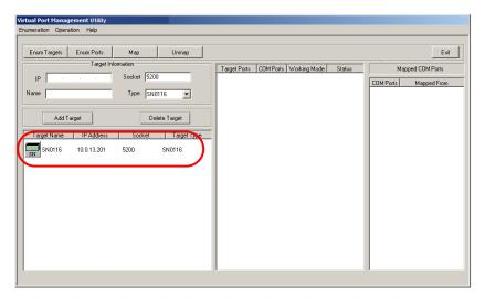
**Note:** Double clicking an item in the list invokes the same function as selecting **Enum Ports**—which displays the numbers and working modes of the selected target's ports in the *Port List* column.
