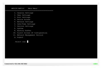
The Main Menu is the text based equivalent of the browser configuration and control functions. The descriptions and explanations for the Browser Operations apply to the submenu functions presented here, as well.
