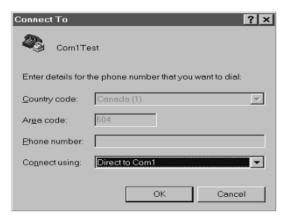
4. For the *Connect using:* field, select *Direct to COM1* (assuming you are using COM1 on your PC), then click **OK**. A *Port Setting* dialog box similar to the one below comes up:
