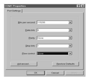
5. For OOBC connections, the SN0108 / SN0116's serial port settings and the computer's COM port settings must be the same. Change the settings in your dialog box (if necessary), so that they match the SN0108 / SN0116's Console Port settings (see Port Config, page 31, for details), then click OK.
