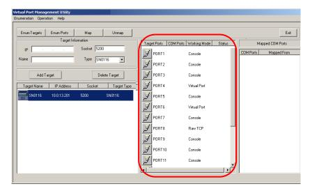
The left column lists the target's port numbers, the second column shows the COM port it is mapped to (if any), the third column shows its working mode, and the right column shows its status.
