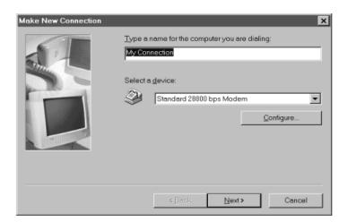
3. Key a descriptive name for the connection in the top text box; select *Standard 28800 bps Modem* for the device; then click **Configure**.
