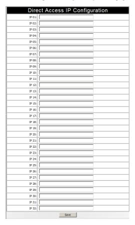
If no IP addresses are specified on this page, anyone can open a TCPIP Telnet session to a RAW TCP or Real COM port by specifying the IP address and port number of the port – without having to specify a Username and Password.
