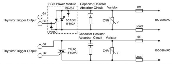
Note: it is recommended to use the SCR power module, which includes a pair of SCRs and diodes. Compared to TRIAC, it is more reliable and consumes less electricity.
