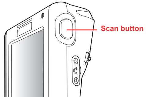
1. To launch Scanner Settings, tap **Start** → **Settings**, and then switch to **System** tab. Tap the **Scanner** icon.
