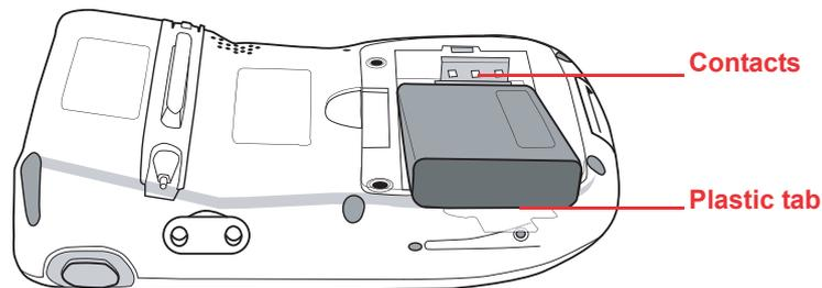
4. Slide the battery pack into the battery bay while simultaneously pulling the battery hook until the battery clicks into place.
