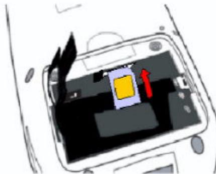
2. Push the SIM card to the end until you hear a click. Push the lock to the right to lock the card by stylus.
