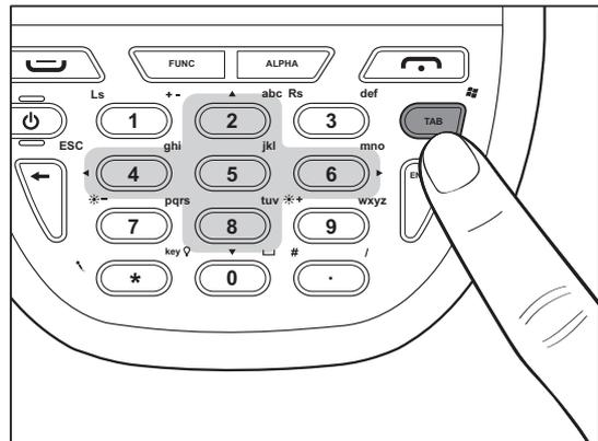
2. While holding the TAB key, insert the tip of the stylus into the reset hold on the back of the PA600. Press and hold the reset button until you see the unitech splash logo screen. Wait 5 seconds and then release the TAB key.
