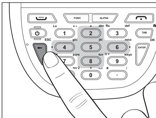
2. While holding the Func key and Backspace key, insert the tip of the stylus into the reset hold on the back of the PA600. Press and hold the reset button until you see the unitech splash logo screen. Wait 5 seconds and then release the Func key and Backspace keys.
