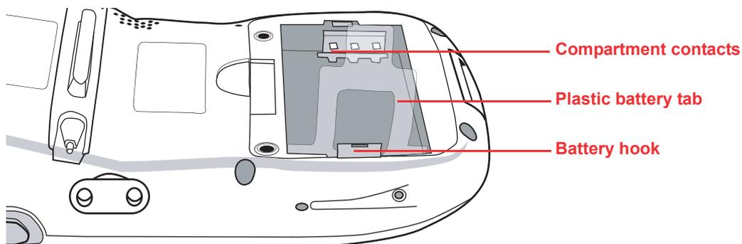
**NOTE:** The plastic battery tab makes it easy to remove the battery.
