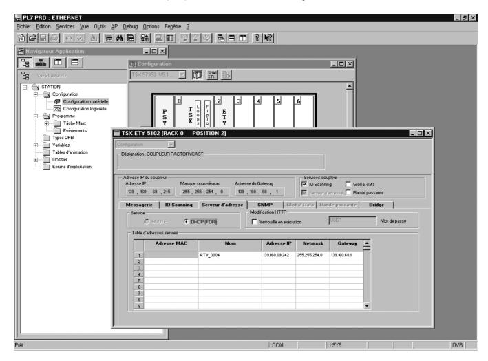
This window is used to configure the DHCP server.
