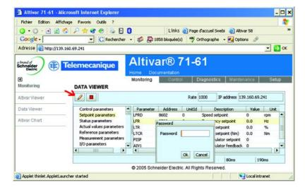
It is only possible to modify the parameter values after entering the "Write password" (see "HTTP password" and "Data write password pages" section on page 54). Click on the "Password" button to enter this password. An entry field then appears in the parameter table, and also a "Cancel" button, for canceling the password entry. After entering the password, press the Enter key so that it is taken into account by the Web browser.
