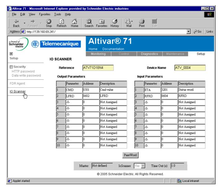
All modifications are protected by the "Write password" modification password. Click on the "PassWord" button to enter the "Write password". After correctly entering the password, you can access "loScanner", "Time Out (s)", "Master", "Output parameters", "Input parameters" and the "Save" and "Abort" buttons.
