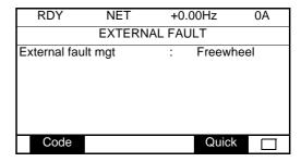
The values of parameters: [COM. fault mgt] ( [ L L ) that will trigger a drive fault [Com. network] ( [ n F ) and [External fault mgt] ( [ P L ) that will trigger a drive fault [External fault com.] ( [ P F 2 ) are: [Freewheel] ( [ E E S ): Freewheel stop (factory setting).
