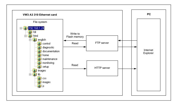
The Ethernet card has an embedded FTP server which authorizes access to the various URLs available for the HTTP server. A browser such as Internet Explorer can be used to display the URLs like a disk in the Windows explorer. This "disk" consists of various directories containing the URL files. It is therefore possible to use the different commands managed by the explorer such as deletion, renaming or writing (downloading) files (check that card IO Scanning has been disabled).
