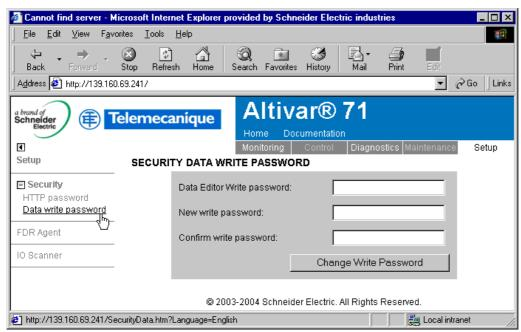
**Note:** Do not lose the user name or the passwords. If they are lost, the Web server can no longer be used, and the card has to be sent for repair.
