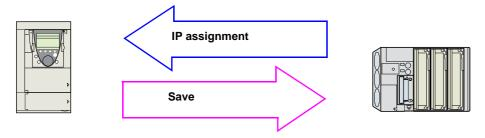
If the drive parameter configuration is local, the FDR server only assigns the IP addresses:
