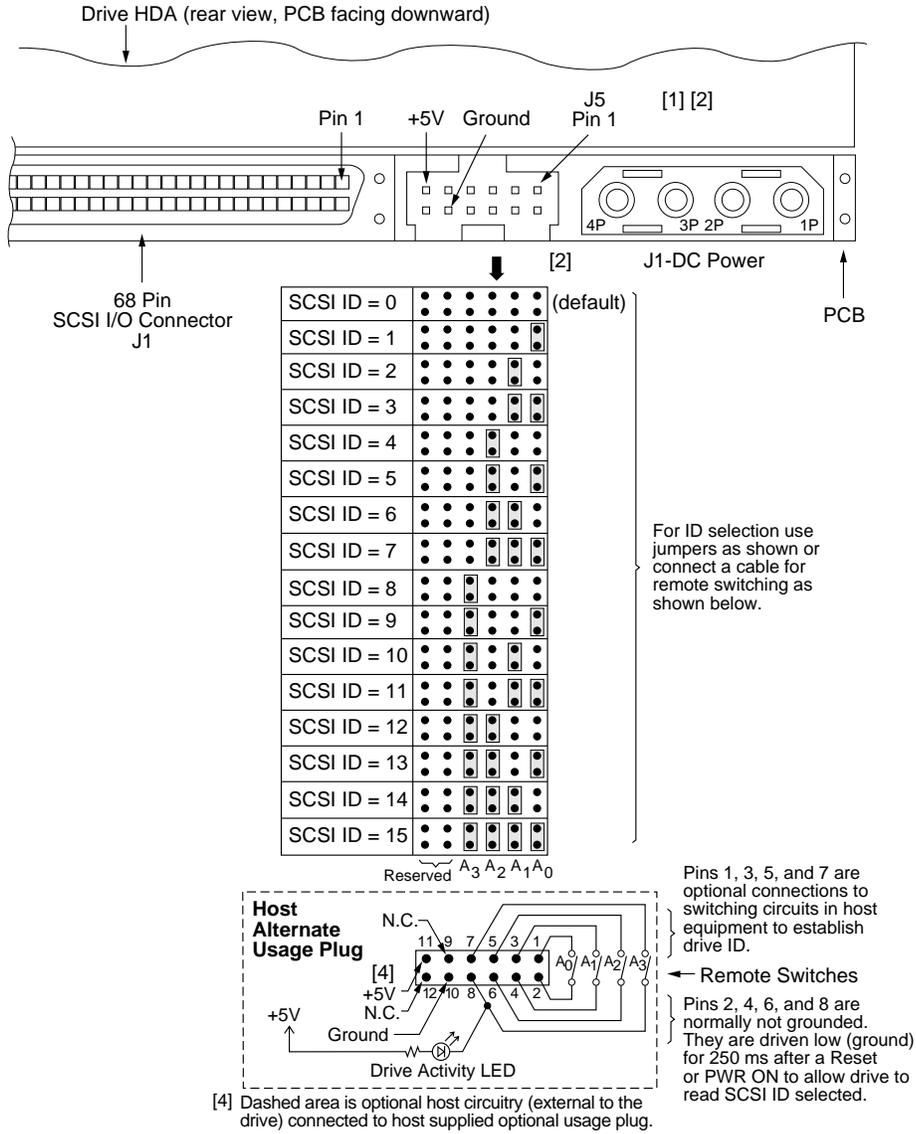
Figure 13. J5 jumper header (on LW/LWV models only)
