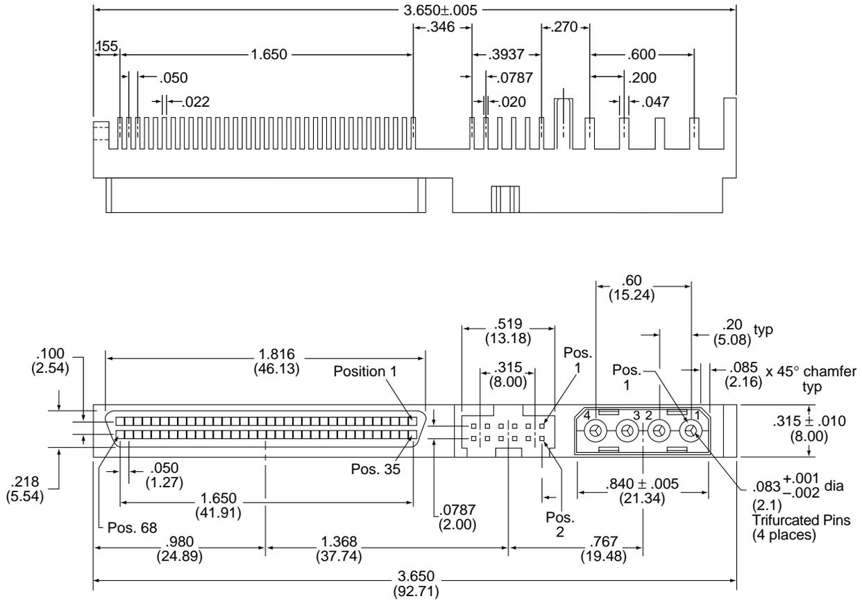
Figure 19. Nonshielded 68 pin SCSI device connector used on LW/LV drives
