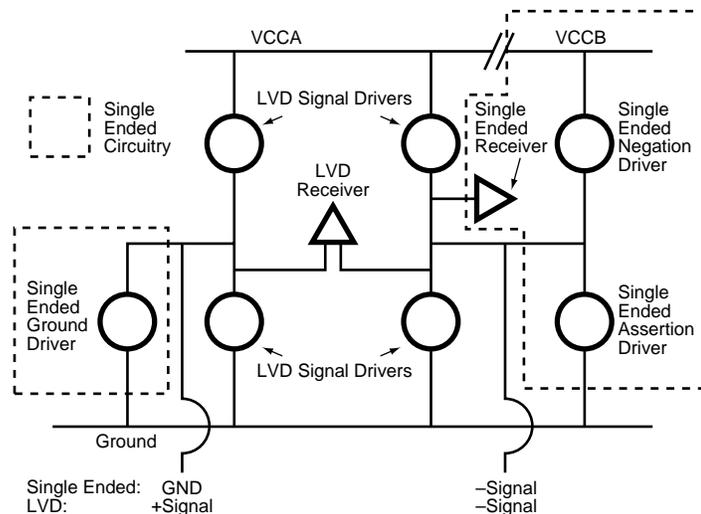
**Figure 22. Typical SE-LVD alternative transmitter receiver circuits**
