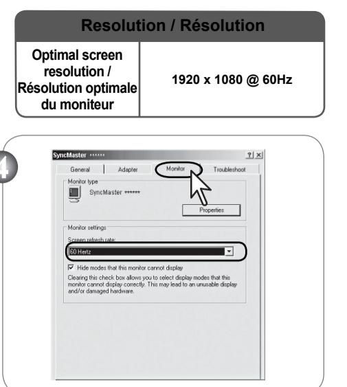
With an PDP monitor, you may experience poor picture quality or noise if the resolution and the frequency are not set to their optimal ranges. Ensure that you adjust the settings as above for the best viewing experience.
