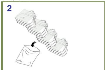
At time of final packing, several pieces of 25cm x 25cm Micro-Pak® Sheets should be used with one sheet placed flat between every two to three bags.
