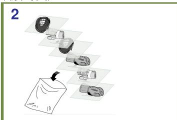
At time of final packing, several pieces of 25cm x 25cm Micro-Pak® Sheets should be placed flat inside the polybag with one piece in between each pair of gloves.
