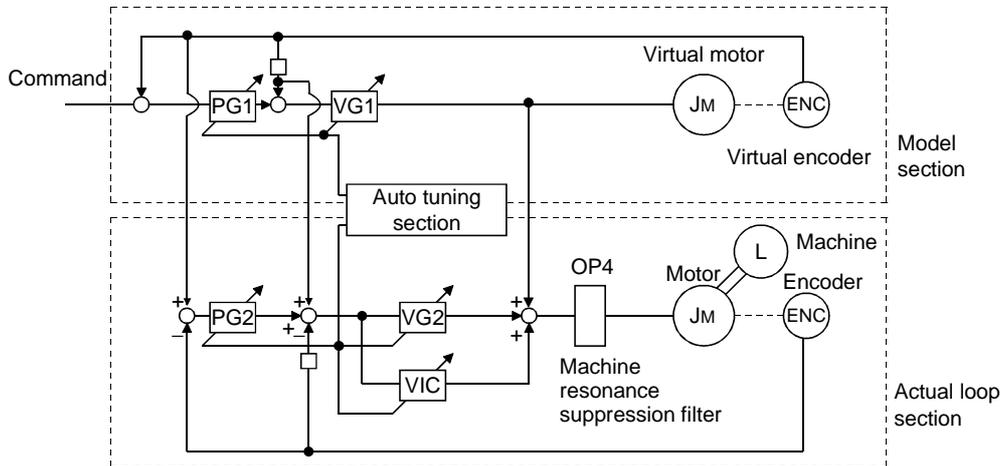
The block diagram of the Servo Amplifier servo control section is shown above. (The current loop is omitted.)
