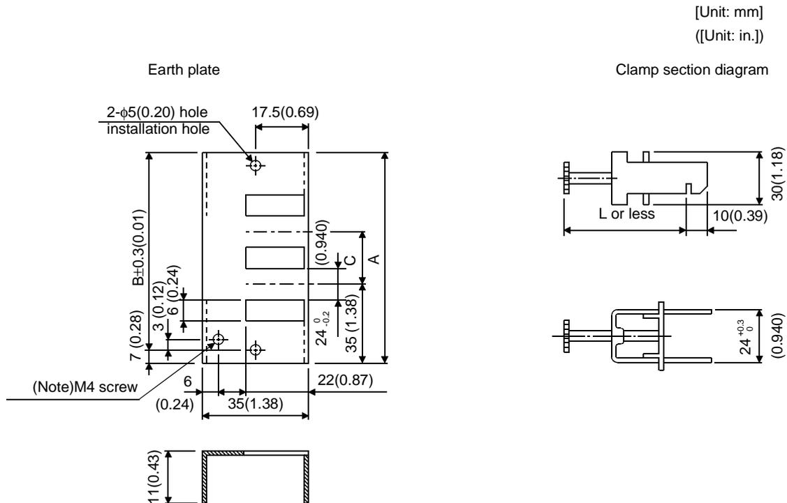
Note: Screw hole for grounding. Connect it to the earth plate of the control box.
