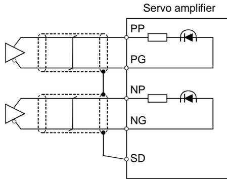
The explanation assumes that the input waveform has been set to the negative logic and forward and reverse rotation pulse trains (parameter No.21 has been set to 0010). For the differential line driver, the waveforms in the table in (a), (1) of this section are as follows. The waveforms of PP, PG, NP and NG are based on that of the ground of the differential line driver.
