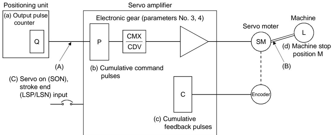
When a position shift occurs, check (a) output pulse counter, (b) cumulative command pulse display, (c) cumulative feedback pulse display, and (d) machine stop position in the above diagram.
