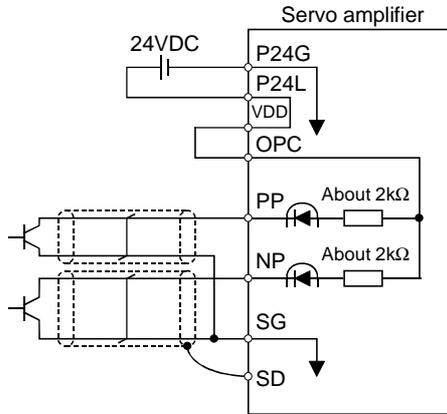
The explanation assumes that the input waveform has been set to the negative logic and forward and reverse rotation pulse trains (parameter No.21 has been set to 0010). The waveforms in the table in (a), (1) of this section are voltage waveforms of PP and NP based on SG. Their relationships with transistor ON/OFF are as follows:
