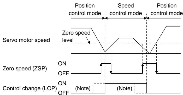
Note: When ZSP is not on, control cannot be changed if LOP is switched on-off.
