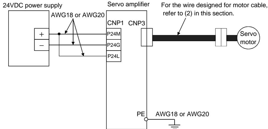
The wires used assume that they are 600V vinyl wires and the wiring distance is 30m max. If the wiring distance is over 30m, choose the wire size in consideration of voltage drop.
