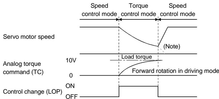
Note: When the start signal (ST1 · ST2) is switched off as soon as the mode is changed to speed control, the servo motor comes to a stop according to the deceleration time constant.
