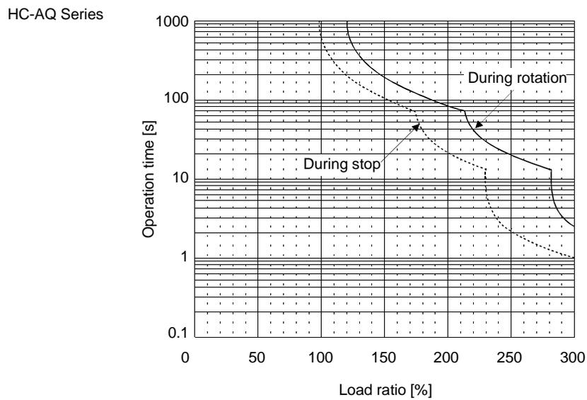
Fig 11.1 Electronic Thermal Relay Protection Characteristics
