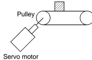
(b) Machine in which a disc is rotated without reduction gear
