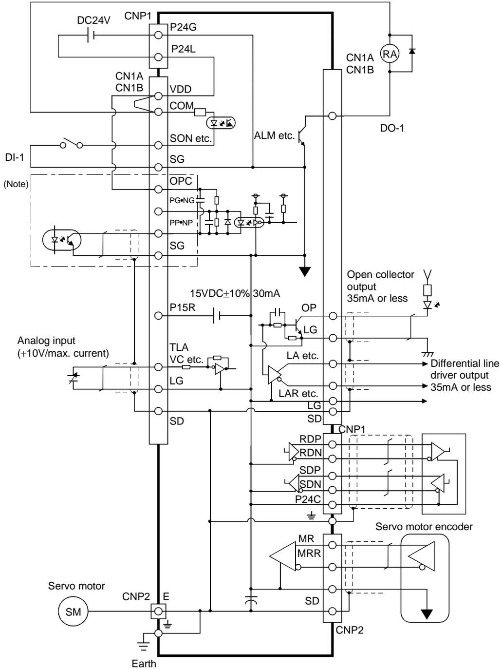
Note: For the open collector pulse train input.
