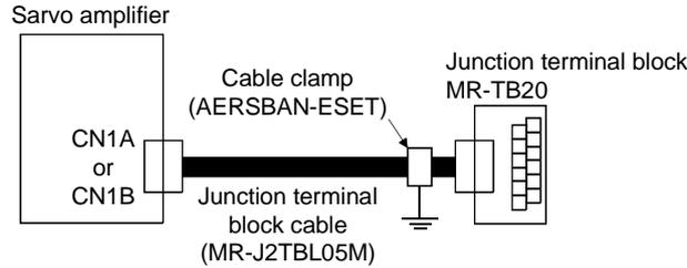
Ground the junction terminal block cable on the junction terminal block side with the standard accessory cable clamp fitting (AERSBAN-ESET). For the use of the cable clamp fitting, refer to Section 12.2.4, (2), (b).
