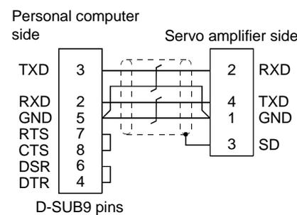
Note: The PC98 Notes having the connector of half-pitch 14 pins are also available. Confirm the shape of the RS-232C connector of the personal computer used.
