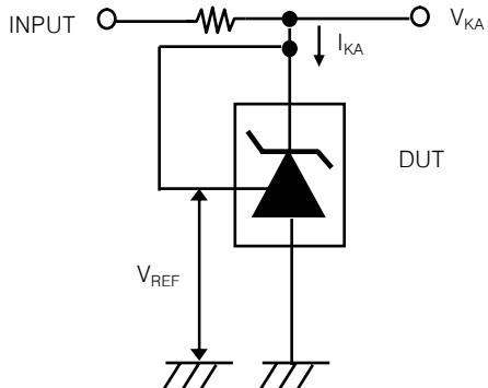
Fig. 2 Test Circuit for  $V_{KA} \geq V_{REF}$
