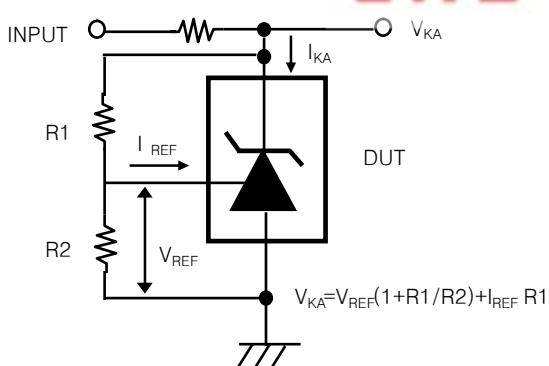
Fig. 3 Test Circuit for  $I_{KA}$  (off)
