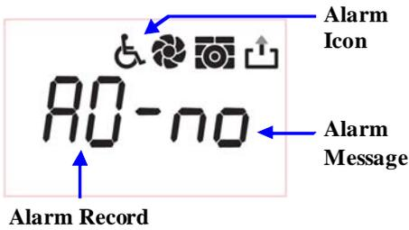
When alarm happened, the LCD display will show message as the figure showed in the left side. If used panel is COLOR type, the display back light will turn to red.
