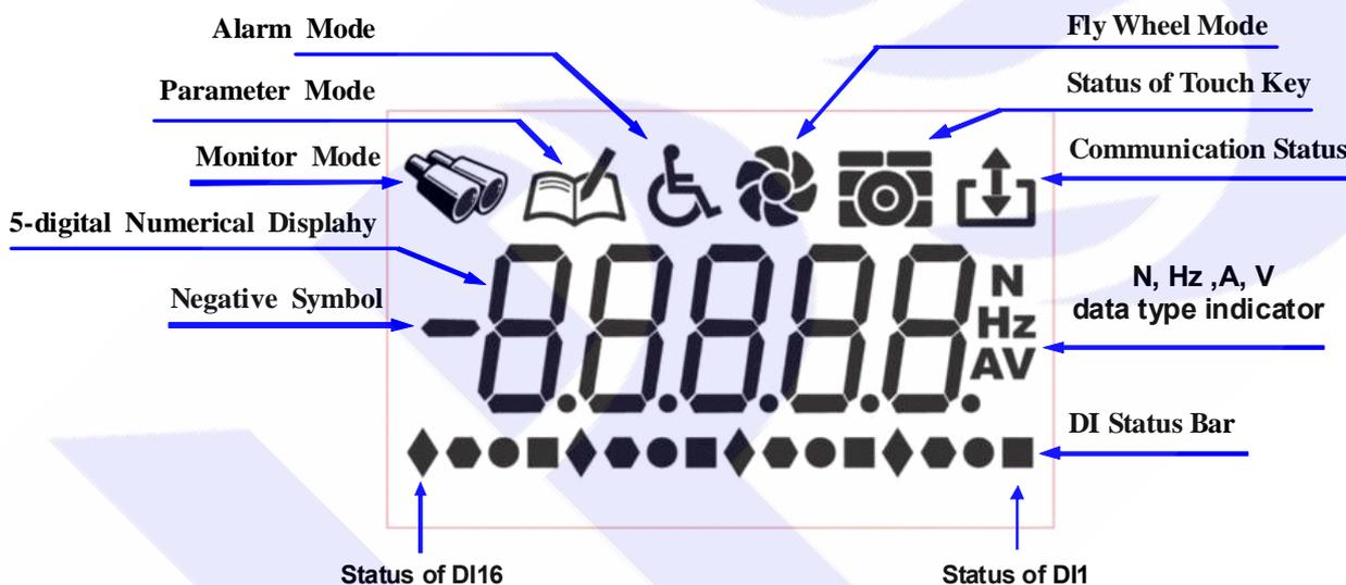
The DI Status Bar shows the on/off status of DI1 ~ DI16 for real time.
