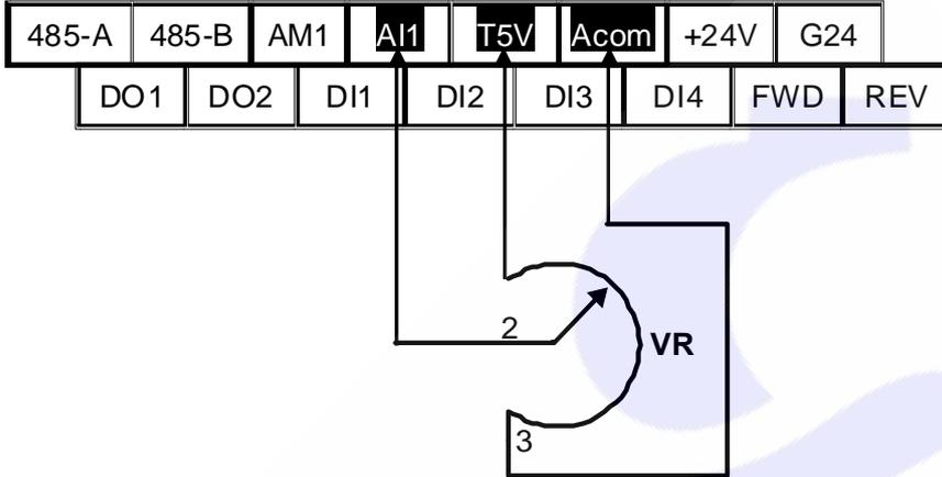
**Example 3: Using external +10V ~ -10V signal as speed command.**
