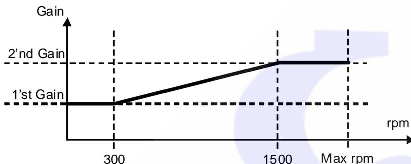
1. When speed start from 0rpm to 300rpm (under the 1'st gain switch point), the driver uses the 1'st PI tuning parameters for close loop control.
