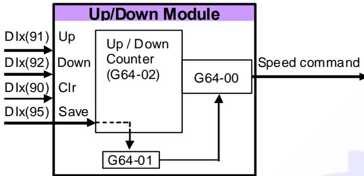
Set all the parameters as the drawing showed in front of here. The start value of Speed Up / Down Counter can be determined by selecting the type of G64-00 to start from 0 or preload a value from G64-01.
