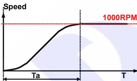
If setting G17-00 (Acc. Time) = 1.00 (Sec/Krpm), and G17-02 (S-curve T1 Time) = 1.00sec, G17-03 (S-curve T2 Time) = 1.00sec.
