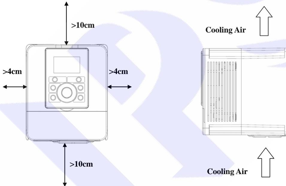
Ensure that the temperature does not exceed the specified level when the inverter is installed in cubicle.
