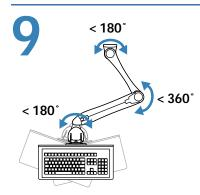
**ARM SWING – Side-to-side:** This product is designed to adjust quickly and easily according to your needs – refer to following steps for adjustment.
