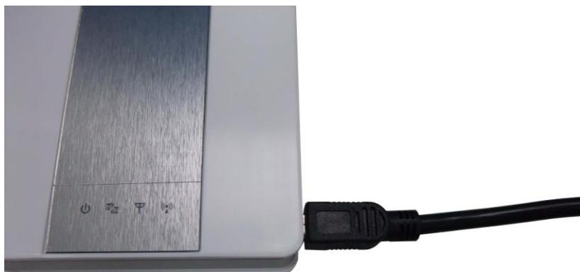
**Step 4.** Then plug the other end of the Mini-USB cable into a PC.
