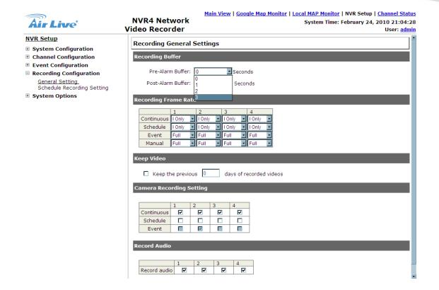
The "recording buffer" allows user to configure the "pre-alarm" and "post- alarm" time for event recordings. The "pre-alarm" time sets the NVR to record in advance when an event is triggered. The "post-alarm" time sets the NVR to continue recording for a period of time after an event trigger is finished.
