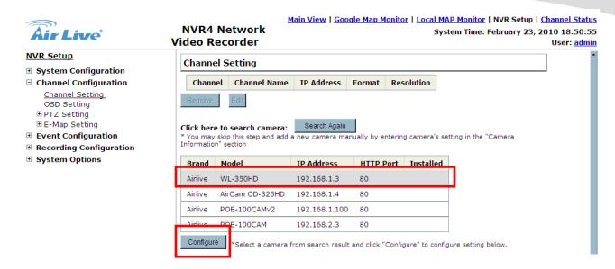
The NVR will retrieve the information about the selected IP camera. The information should be displayed on the "Camera Information" section. Enter the username and password of the IP camera, then select the channel ID and name the camera.
