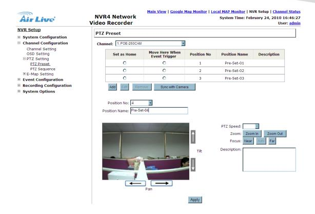
**a.** To set up PTZ preset points, select a camera from the "Camera" drop-down menu and click "Add".
