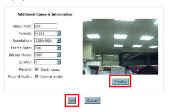
Adjust the video format, frame rate, resolution or bitrate... according to your environment. You can also click on the "Preview" button to preview the live video of the camera. Click "Add" to finish adding the camera.
