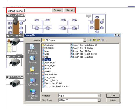
**b.** Then drag and drop the camera icon to define its location. Then press the "Apply" button
