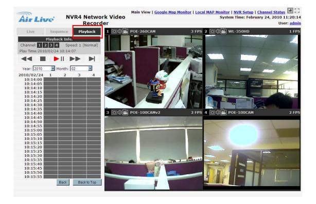
Playback is a function that allows you to play one or more videos that were previously recorded by a chosen recording method or due to an event trigger. The NVR offers synchronized playback from up to 4 channels and various types of search methods are provided to help you find the footage you need quickly.
