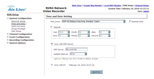
Set the time and date by selecting the time zone according to your location. It is imperative that you set the NVR's time correctly to avoid the following errors:
