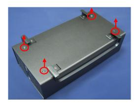
• Push the inner enclosure out, and remove the outer chassis.
