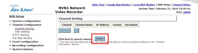
After that, the NVR should begin to search the IP camera and the progress of the searching should be displayed on the screen:
