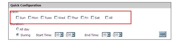
**c.** You might set the duration separately via the "Start Time" and "End Time" drop-down menu, or select the "All day" option to make the NVR recording for 24 hours.
