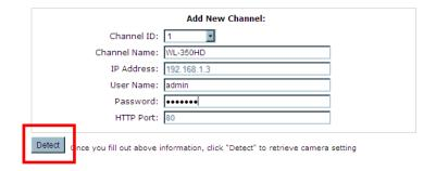
Click on "Detect" button for establishing the connection between the NVR and the camera. If connection establishes, the detailed information of the IP camera should be polled and displayed as below
