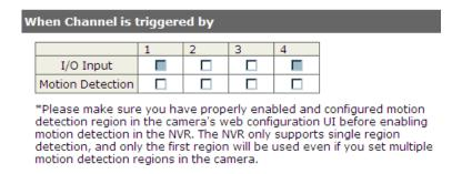
**b.** Use the checkbox to enable system event trigger. The system events are list as below:
