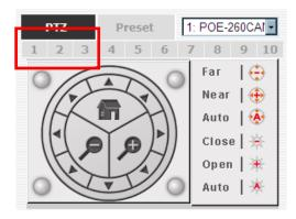
Camera(s) that are currently being selected for live viewing will be listed in the PTZ drop-down menu. Simply select a camera then use the PTZ control panel to control the camera
