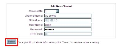
Click on "Detect" button for establishing the connection between the NVR and the camera. If connection establishes, the detailed information of the IP camera should be polled and displayed as below
