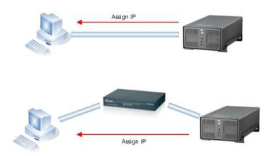
The PC that is connected directly to the NVR (or within the same local area network) should receive an IP from it. Simply access the NVR from your web browser with its IP address
