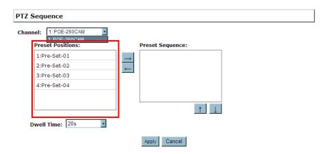
**c.** Pick the ones you like for sequence viewing and press the "->" button to move them to the "Preset Sequence" section, then use the up and down buttons to adjust their sequencing positions.
