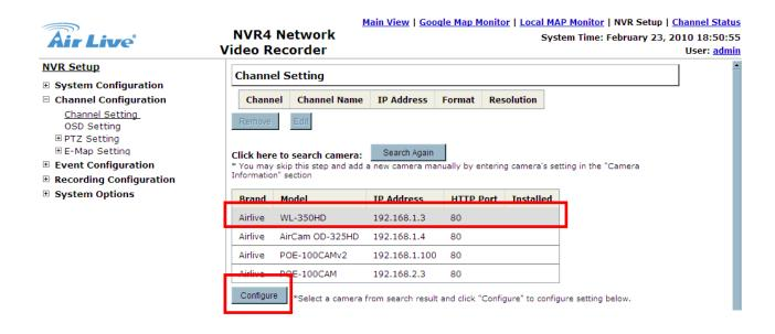
The NVR will retrieve the information about the selected IP camera. The information should be displayed on the "Camera Information" section. Enter the username and password of the IP camera, then select the channel ID and name the camera.
