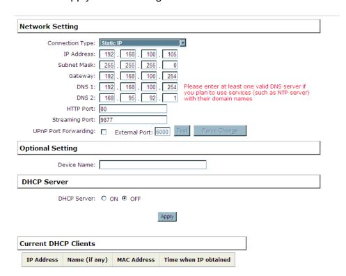
Note: The NVR can detect the presence of a DHCP server upon startup. It sets itself to use
