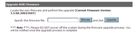
**Note:** During the upgrading process, please do not unplug the power or the network cable from the NVR, for that will damage the NVR and raise the reparation issue. Besides, after upgrading the firmware, you will not be able to downgrade to the previous version. Please contact your dealer or installer for the firmware upgrade operation.
