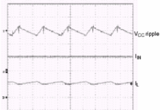
Figure 25. Boost Input Voltage and Current Ripple Waveforms
