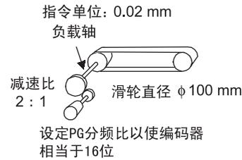
$$\text{负载轴旋转1圈的移动量} = \frac{3.14 \times 100 \text{ mm}}{0.02 \text{ mm}} = 15700$$
