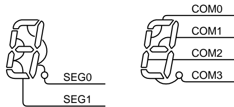
Figure 16-6 Example of COM, SEG Pin Connection (1/4 Duty)
