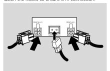
2 Connect the passive subwoofer to the SUBWOOFER (8Ω) terminal with the supplied subwoofer cable by matching the plug types.
