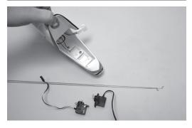
12. Pull and twist tail boom out of fuselage after slicing white boot where it connects tail boom to fuselage. This step requires moderate force.
