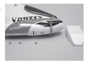
3. Unscrew the front servo's front screw (don't remove rear screw).
