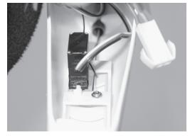
9. Unscrew bolt holding in the tail boom at rear of fuselage.
