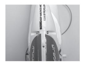
20. Follow steps 1-7 in reverse order to re-assemble Vortex completely (Rear servo first: Z-bend on servo arm, servo in servo mount, front screw. Repeat for front servo. Connect servos to receiver. Three servo mount screws. Foam battery holder.).
