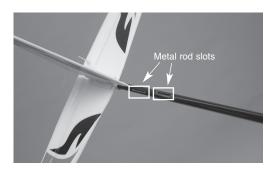
14. Push the new tail boom into the fuselage. The front of the tail boom should be about 1/4" past the tail boom former.
