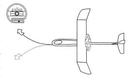
• Fly in a straight and level line: To do this the wings must be level and the throttle must be in the correct position on the transmitter. Use small movements with the right stick to hold the wings level, and experiment with the elevator to find out where it must be for level flight.
