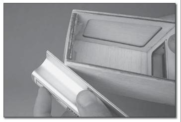
□ 2. Lightly sand the forward part of the fuselage where you will apply the fiberglass. Round the edges of the fuse sides slightly. Use compressed air or a tack cloth to clean any dust from the fuse before you begin glassing.
