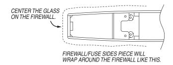
□ 6. Mix up another batch of finishing resin and brush a thin coat onto the firewall and forward fuse sides. Center the 3-1/2" x 20" [89 x 508mm] piece of glass cloth on the firewall and wrap it around to cover the fuse sides. Stipple and squeegee the glass cloth smooth. Allow the resin to cure and sand the fiberglass smooth.
