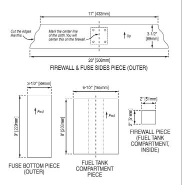
□ 1. Cut out the following pieces for the fuselage from 3/4oz [21g] fiberglass cloth:
