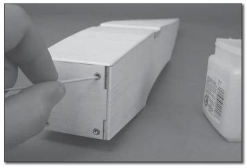
$\Box$  4. Fill the threads of the blind nuts with petroleum jelly using a toothpick.
