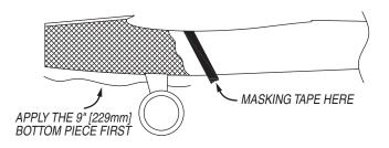
□ 5. Mix up about 3/40z [22cc] of finishing resin. Brush on a thin coat of resin to the bottom of the forward fuse. Apply the 3-1/2" x 9" [89 x 229mm] rectangular piece of fiberglass to the bottom of the forward fuse. Align the forward edge of the glass with the edge of the firewall. Stipple the glass cloth down to the fuse. Squeegee any excess resin out of the glass so that the surface is smooth. Allow the resin to cure. Sand the fiberglass smooth feathering the glass into the balsa.
