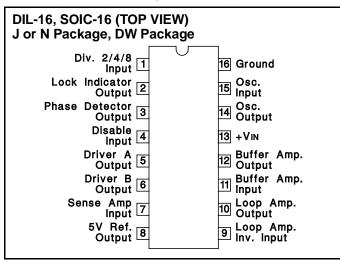
Note 1: Voltages are referenced to ground, (Pin 16, DIL Package). Currents are positive into, negative out of, the specified terminals.
