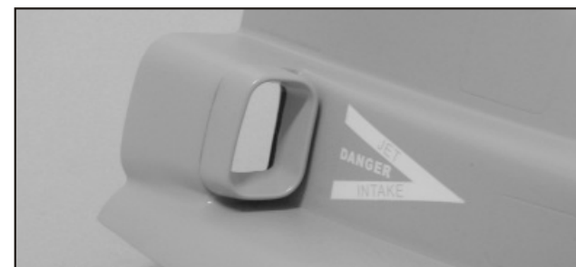
92. Epoxy the Air Inlet assembly to the fuselage. Do the same on the other side.
