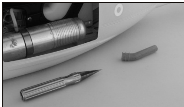
59. Drill a 10mm hole for diverter out of the bottom fuselage.
