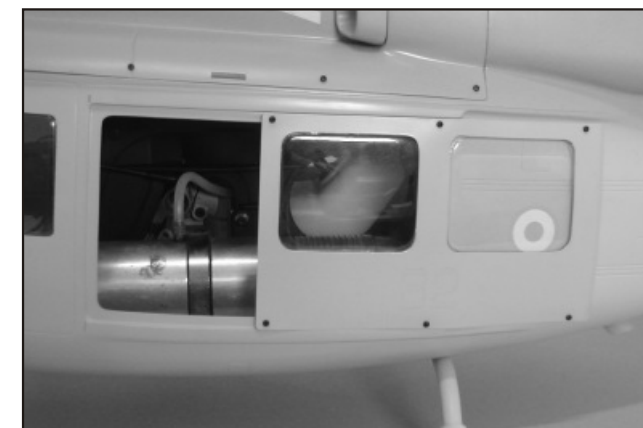
118. Use the hole on sliding door as the guide to drill 1.5mm pilot holes on the fuselage. Suggest to do an "open" door as photo shown, it will be easier to access the fuselage to maintain the mechanism also get a better cooling in flight. Secure the door with six 2x5mm wood screws.
