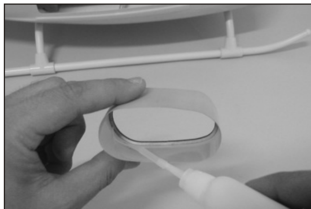
99. Glue the frame in place and make sure it is flush with the opening.
