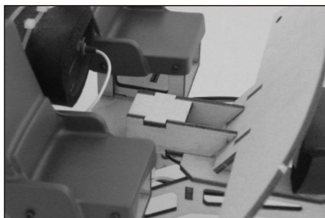
110. Glue the whole cockpit wood structures in place as photo shown. Includes seats, instrument panel and center control panel.
