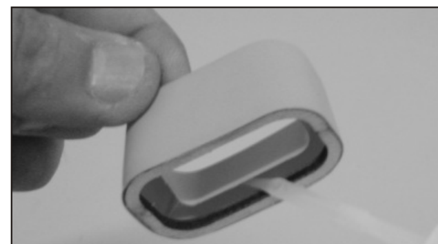
91. Glue the reinforced frame inside the Air Inlet. Note the frame must be flush with the opening.
