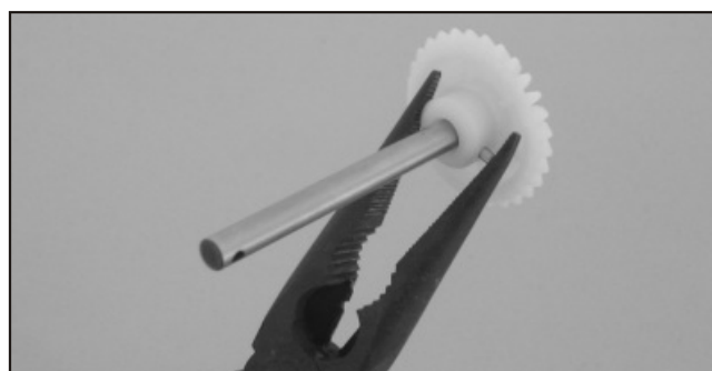
34. Install the bevel gear on the long shaft with the pin.
