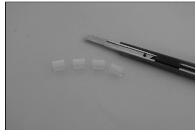
51. Locate a silicone tube then cut to four pieces as photo shown.
