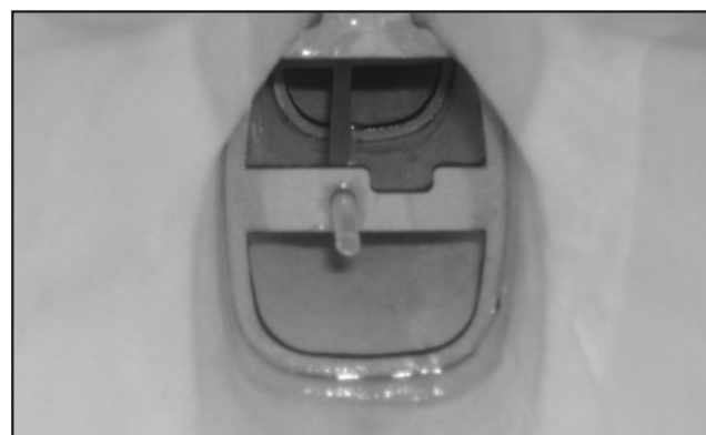
48. Same way to install the other tail bulkhead in place. The tube is only 35mm in length off the bulkhead.
