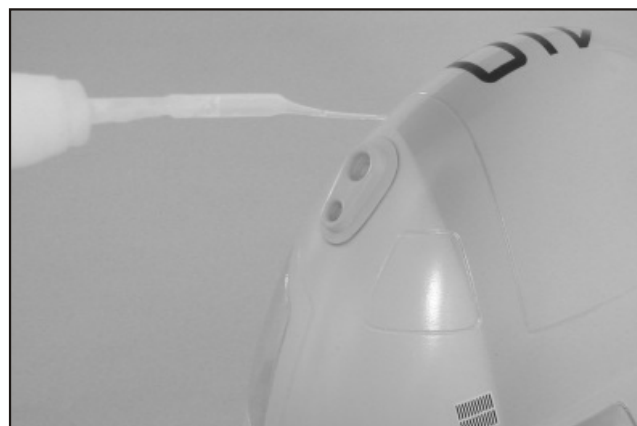
8. CA the navigation light in place as shown.
