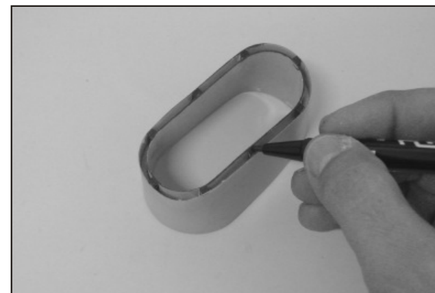
103. Use marker to paint the spacer in dark for scale looking.
