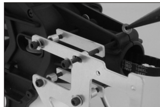
38. Install rear frame on the Titan with furnished the aluminum doublers, standoff. Do not secure at this moment. You will need four 3x45mm socket screws, eight standoffs, eight M3 washers, four M3 locknuts and two doublers.
