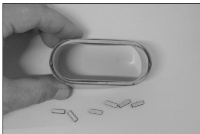
101. Locate the spacer from the plywood sheet C and glue them averagely between inner vent and outer vent.
