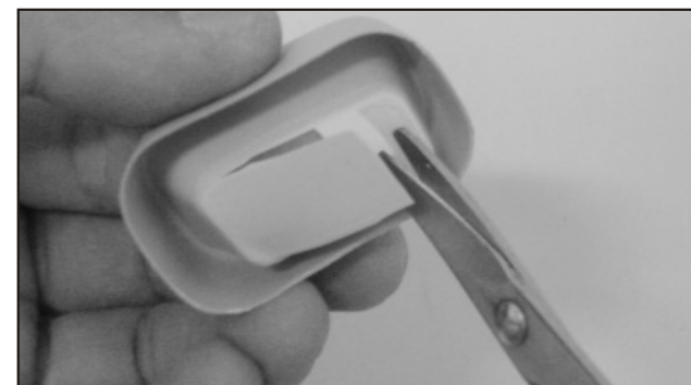
90. Trim the inlet with curve scissors.
