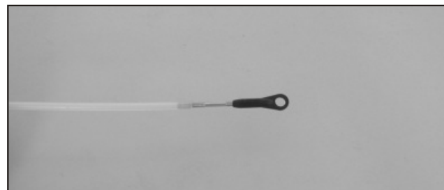
49. Install the flexible tail pitch pushrod. Thread the straight threaded rod into the tube and ball end as shown.
