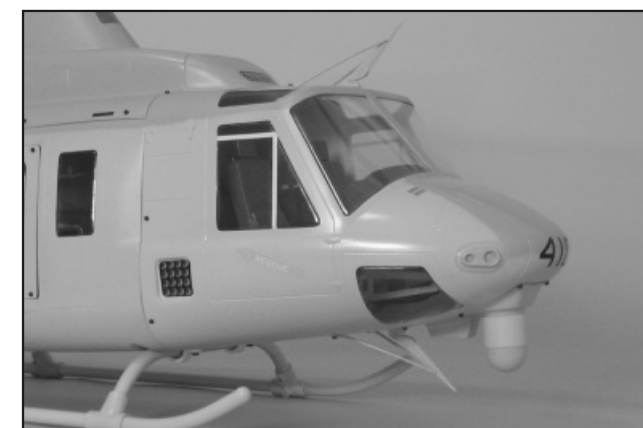
119. You may do the same "open" door on the other side or do it a "close" door. Trial fit the front fuselage in place and drill six 1.5mm pilot holes. Secure the front fuselage with 2x5mm wood screws.
