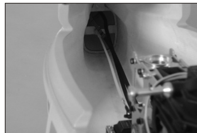
65. Install the mechanism in the fuselage again, thread the belt through the fuselage and the pushrod through the guide tube.
