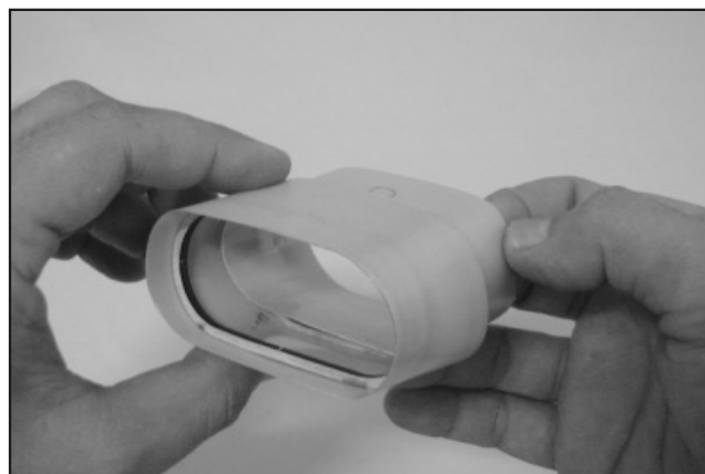
100. Glue the other reinforced frame in the outer vent, note the distance to the edge is about the length of plywood spacer as you can see in the next photo. Trial fit the inner vent in the outer vent.
