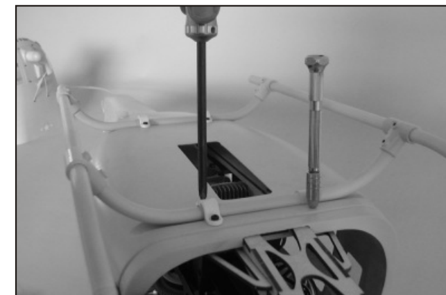
66. Secure the mechanism on fuselage with 3x18mm wood screws.
