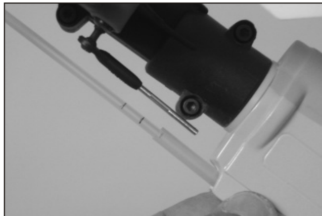
85. Measure the flexible pushrod, consider the control throw of the control lever and at least about 6mm threaded rod inside the pushrod then carefully cut away guide tube first then the pushrod. Note the pushrod and guide tube might not at the same length, do not hurt the inside pushrod.
