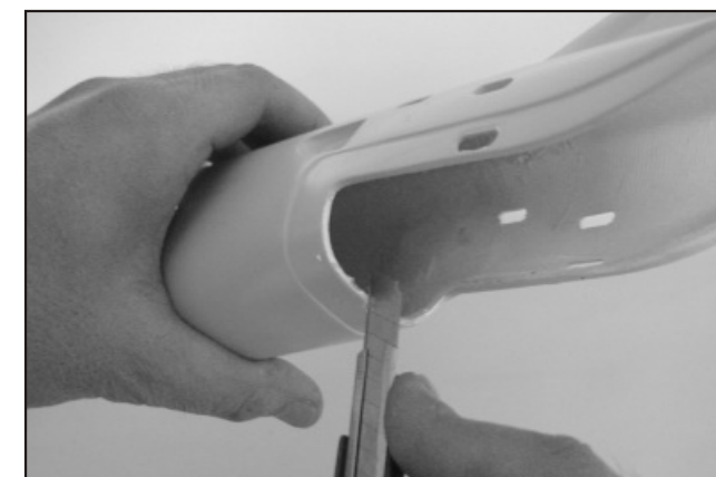
42. Trim the tail so the support mount assembly could fit inside perfectly.
