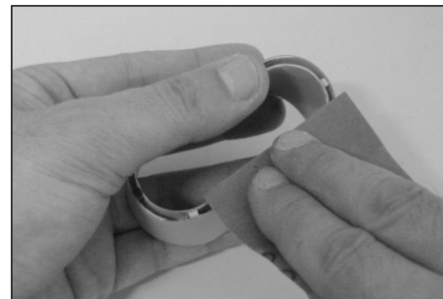
102. Sand two opening and make sure they are level at the opening.
