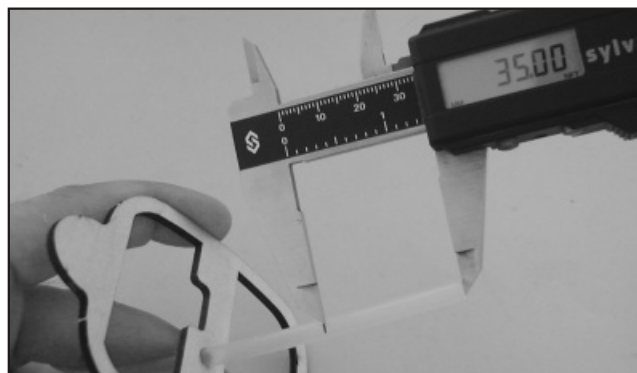
46. Thread the guide tube to the other bulkhead as shown and leave 35mm in length off the bulkhead.
