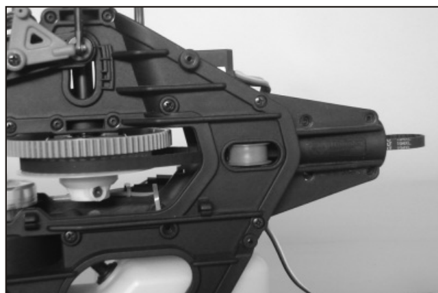
32. Remove the tail boom and old belt. Install the new short belt as shown.
