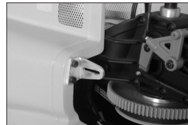
67. Secure the retainer on post and make sure fuselage is not binding.
