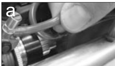
a. Pinch fuel tube to stop fuel flow.
