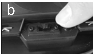
b. After stopping the engine, turn off the receiver switch first, then the transmitter.
