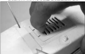
33. You will have to bow the cover plate to close or pry with finger to remove the cover plate. Note the opening is forward to the nose for battery cooling.
