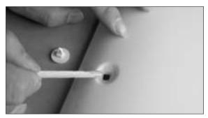
3. For novice, we would recommend to epoxy one strut mount at one time. Note the orientation
