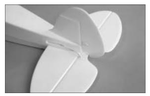
13. Trail fit the horizontal tail and vertical tail in the fuselage, epoxy the them in place when satisfied. Make sure they are perpendicular to each other.
