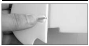
11. Locate the control horn and locking plate then "Push-N-Lock" the control horn in place as shown. Note: Do not push too hard but gently all the way in so the control horn contacts the surface of rudder at both sides and secured in place firmly.
