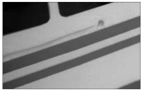
31. Drill a small hole on the fuselage at right side then thread the antenna through the fuselage. Route the antenna to the tail and tape it in place.
