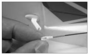
27. Adjust the small clevises and make sure all the control surfaces are level.
