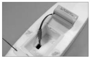
32. Connect the wire to controller and place the battery in the battery case.
