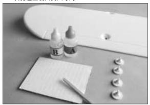
Mix the furnished 5-min Epoxy to glue the strut mount. Hint: Apply equal volume of cement in bottle A and B on a cardboard then fully mix them with a small stick. Note: This 5-min Epoxy allows working time is only 3 minutes after mixing.
