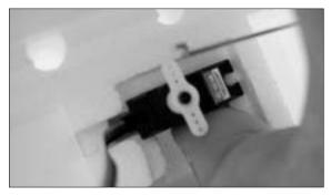
24. Remove a foam spacer from the servo well. Glue the micro servo to the wall of servo well.
