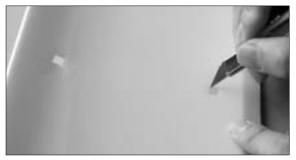
Carefully trim the strut mount hole in square then trail fit the strut mount in the hole. Make sure the strut mount is level with the wing surface.
