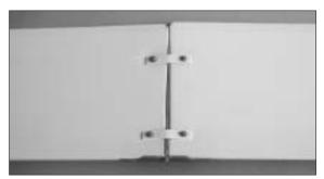
Apply 5-Min epoxy at the contact area then place the two wing halves again and snap on the wing joiners.
