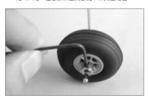
18. Use furnished Allen Wrench to secure the collar in place with 3x3mm set screws. Make sure the wheel rotates freely.
