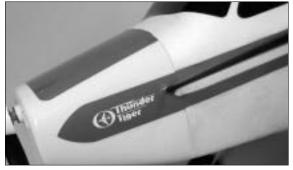
22. Apply cowl decals first then secure the cowl in place with two 2 x 8 mm wood screws.
