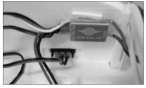
28. Connect the motor wire, next attach the controller( ESC-10 Shown) on the wall by using the double side foam tape. Next, install the controller switch.
