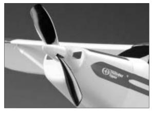
35. Next install the propeller and spinner, always take great care on the motor and swinging propeller as it is dangerous and may cause serious injury, if you are a beginner we recommend you read the manual of radio and speed controller thoroughly to understand how to set up and control the motor.
