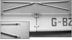
Glue the struts to the Y joiner( one long, one short). Note the orientation of hook opening and the upper tube is shorter as photo shown.
