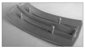
Locate the wing center cover, use 100 grit sand paper( not furnished) slightly sand the contact area of center wing cover.
