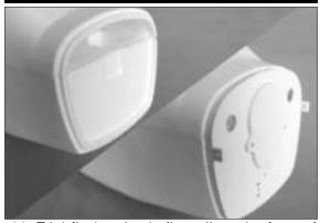
14. Trial fit the plastic firewall on the front of fuselage. Apply Epoxy at the rim of front fuselage then glue the firewall in place.
