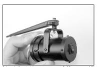
9.Locate the strut A, washer, spacer, 3x22mm screw, M3 locknut and the lamp housing. Next install the strut A on the lamp housing with 3x22mm screw, washer and M3 locknut as shown.
