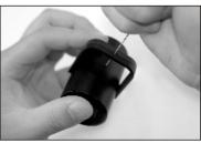
4.Drill a 1.5mm(1/16") hole on the housing through the suspension then enlarge the hole to 3.5mm(9/64") for extension wires.
