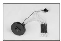
2. Press the switch complete with LED lights into the end cap after heating treat the shink tube in place.
