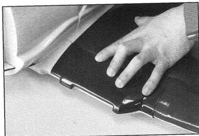
45. Properly glue the radiator inlet at the leading edge where close to the wing root. 以瞬間膠固定冷却器於翼根前緣上。
