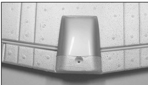
34. Carefully trim and epoxy the radiator scoop in place. 如圖修剪並以環氧樹脂膠合偽裝潤滑油散熱器。
