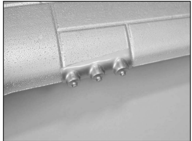
35. Trim and epoxy the machine gun in place, same procedure on the other one. 如圖修剪並以環氧樹脂膠合偽裝機槍孔。
