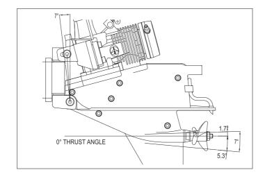
This adjustment is used to alter relationship of the thrust angle to the centerline of your hull, which affects both the speed and attitude in which your boat performs, i.e. bow high, bow low, etc.
