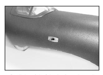
40. Install the switch of the electric speed controller.
