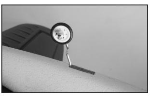
35. Install the tail gear with epoxy in the aft section of the fuselage.
