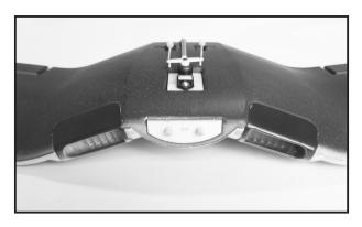
33. Trim the radiator inlet and lightly epoxy them in place. Note the orientation of the inlets. 裁剪冷却器道氣孔,并用環氧樹脂膠合于主翼上。
