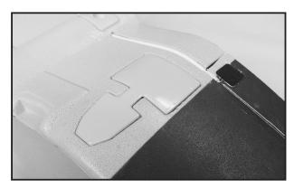
32. For less drag or user desired speed flight, the foe retract gear is a good choice. Trim the vacuum formed foe retract gear as shown and locate them at the bottom wing.
