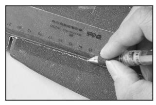
22. You may use a ball pen to draw hinge line then flapping aileron. Make sure the aileron move freely and will not come off.
