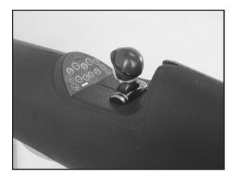
9. Apply the instrument panel decal and the pilot in place.
