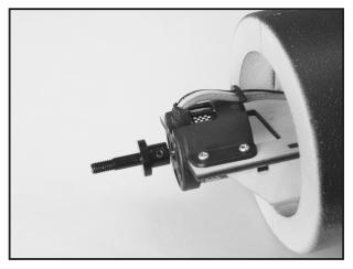
19. Install power unit on the motor mount with 2. 6x8mm wood screw, then secure the adaptor with 3x3mm set screw.
