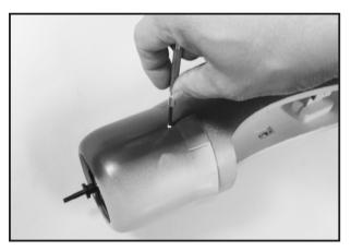
37. Trial fit the cowling onto fuselage then secure with two 2x8mm wood screws at the molded dot.
