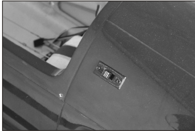
76. Install the switch harness as shown.
