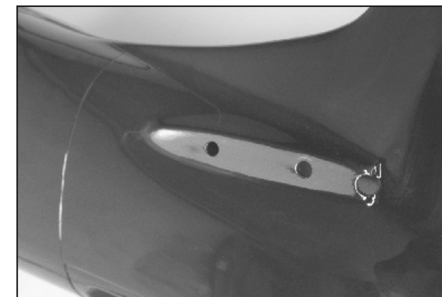
38. Sand the glue area of the fuselage to increase the roughness.
