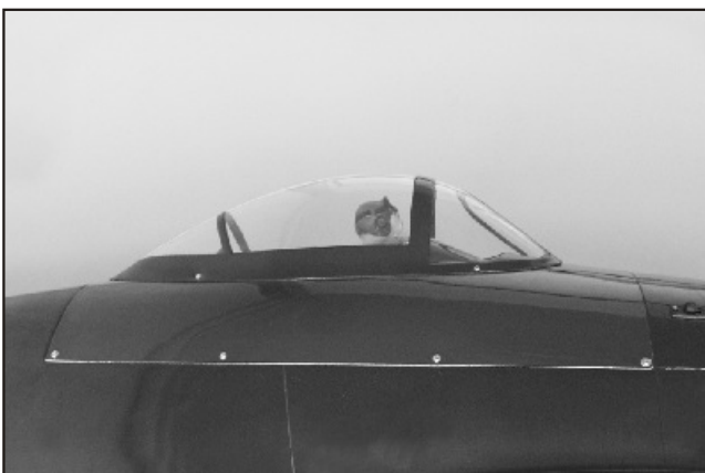
81. Trial fit the upper fuselage cover in place, drill eight 1/16" (1.5mm) holes and glue small plywood doublers inside the fuselage at the holes area. Drill the doublers again and secure the upper cover in place with 2x8mm washer wood screws.
