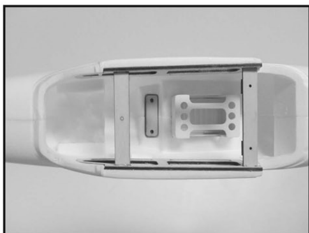
9. Epoxy the landing gear mount and wing mounts.
