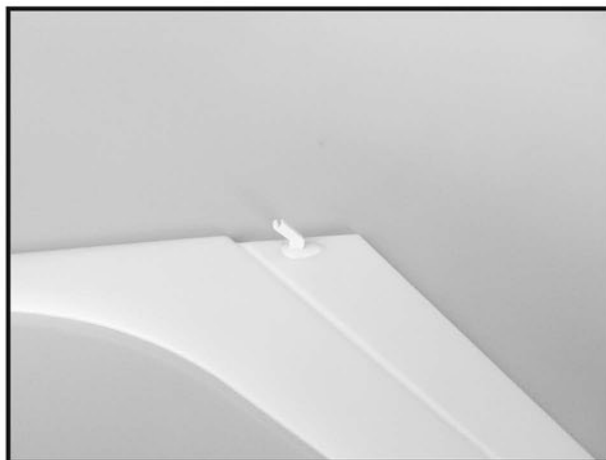
22. Install the rudder control horn. Make sure the orientation of the control horn before you press the backplate,
