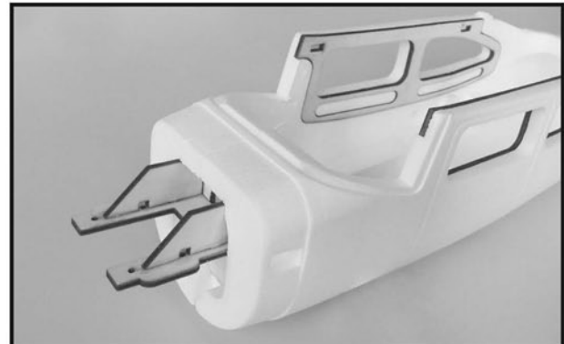
5. Next trial fit the two fuselage halves with firewall. Note the orientation the firewall and make sure two fuselage halves could contact each other closely. Next lightly epoxy two fuselage halves together.
