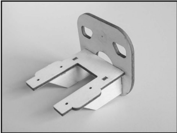
1. Locate firewall, motor mount and mount supports. Epoxy the mount and supports on firewall.
