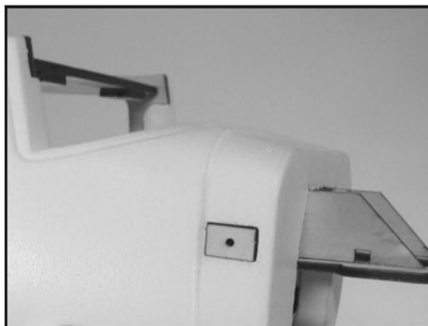
10. Locate the cowling mounts then epoxy the mounts in place.
