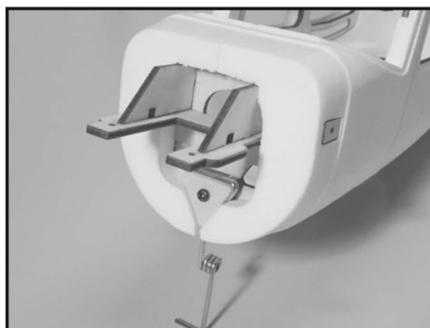
12. Apply enough epoxy and glue the Nose Gear in place with another Nose Gear Mount A. When cures, secure the nose gear assembly with 3x18mm wood screw.
