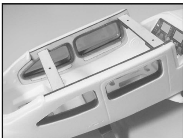
33. Light epoxy the flange of the side windows, then glue them in place.
