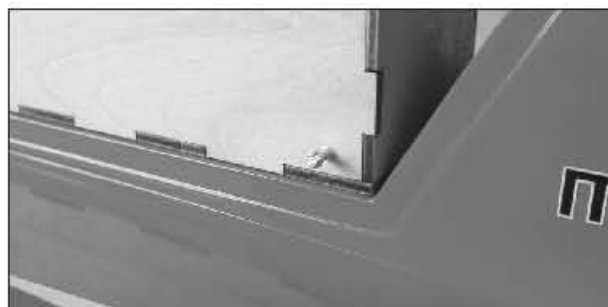
17. Remove the upper deck from the hull. Screw in the retaining posts at the holes you drilled.
