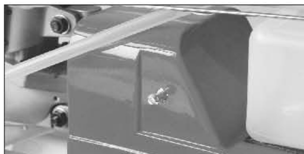
16. Trial fit the upper deck on the hull, use mask tape to tape it in place. Drill 3mm hole at the molded dots at both two sides and deeply into the hull.
