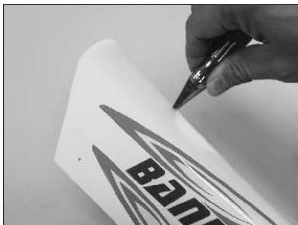
18. Drill the antenna guide tube hole on the upper deck at the molded dot.
