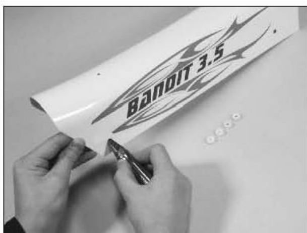
19. Use reamer to enlarge the hole up to 7mm in diameter. Install the grommet in place.
