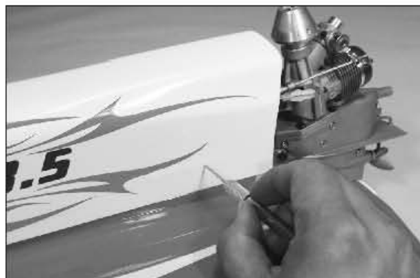
16. Trial fit the upper deck on the hull, use mask tape to tape it in place. Drill 3mm hole at the molded dots at both two sides and deeply into the hull.
