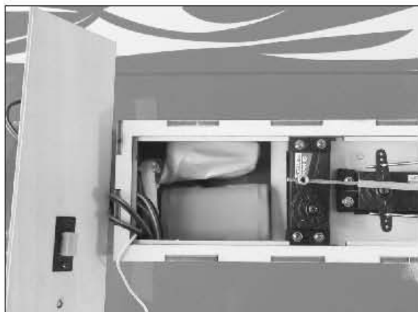
13. Connect all wires properly then install the receiver inside the balloon, use tape or small rubber band to seal the opening. This will help to protect the receiver in case of flipping. Do the same way to the battery case. Suggested to add weight about 100g-130g in radio box case, this is will help the hard turn in the water.
