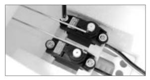
38. See the servo manual and install the eyelet and grommet then secure the micro servos in the servo tray with the wood screws that comes with the servo.
