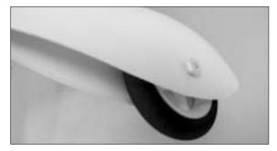
29. Install the wheel pant and wheel on landing gear next thread the plastic nut. Make sure wheel rotates freely.
