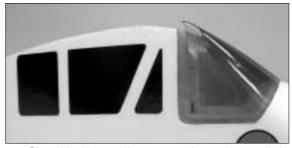
45. Glue it in place with epoxy and note the notch is in line with the wing saddle so the leading edge of the wing could go in.
