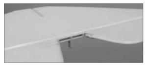
18. Trial fit the joiner in place next apply epoxy and glue it firmly in place. It will be easier to bend two elevators then slide the joiner on the elevator.
