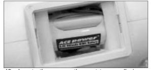
42. Locate the sponge then cut two small pieces and use as spacer to keep battery in case firmly.
