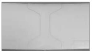
47. Glue the wing center cover in place with epoxy.
