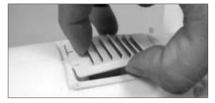
43. You will have to bow the cover plate to close or pry with finger to remove the cover plate. Note the opening is facing to the tail.
