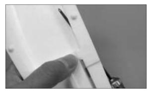
5. Drill 3mm rudder pushrod exit hole at the right fuselage tail. A small amount of angle will give best pushrod performance.
