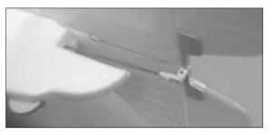
19. Locate elevator pushrod(the short one), insert the pushrod from front fuselage through the pushrod support and exit at the tail. Thread the clevis then snap onto the elevator joiner.
