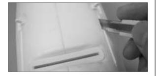
25. Carefully cut the slots at the bottom fuselage about 10mm(3/8") in depth.
