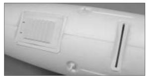
10. Locate the battery box and landing gear mount next epoxy them in place as shown.
