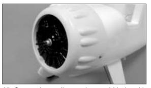
35. Secure the cowling on the wood blocks with three 2x5mm wood screws.
