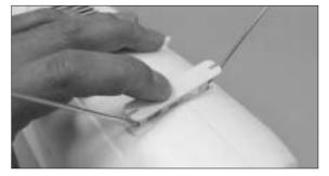
26. Insert the landing gear in the landing gear mount then press the retainer all the way in to secure the landing gear in place. When pressing make sure to support from the inside of fuselage.
