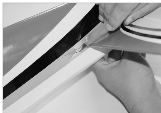
17. Same way to locate the rudder and elevator servo well. Cut an "X" at the servo well.
