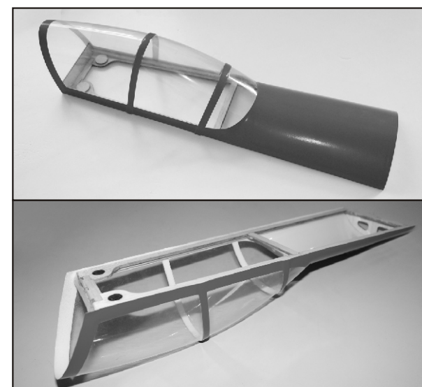
34. Locate the canopy & its frame, trial fit the frame in place. Make sure to leave about 3/32" (2.4mm) at twp sides. Note the front of frame should even with the canopy. The rear canopy should contact the turtle deck smoothly after gluing the frame.
