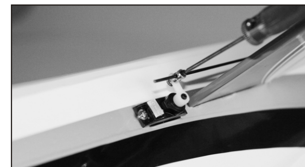
23. Secure the rudder servo at the right side of fuselage with 12" extension wire installed. Adjust the pushrod when servo and rudder are both in neutral position.
