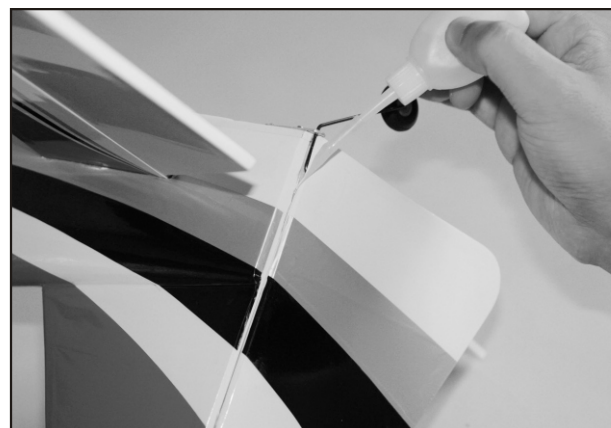
16. Trial fit the rudder in place, make sure it works fine then apply epoxy at the rudder torque rod hole and slot then attach the rudder on the fin. Wipe away the excess epoxy and make sure rudder works freely after cured.
