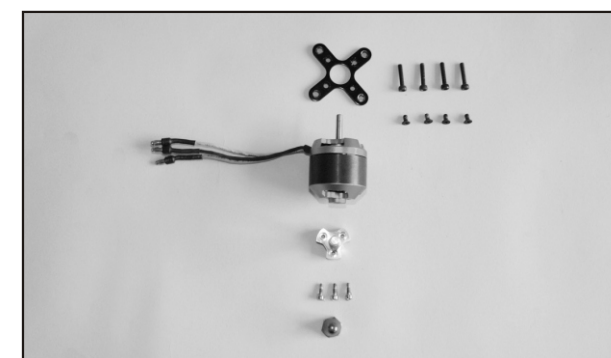
24. Locate the brushless motor, cross mount, adaptor, prop nut and mounting screws if user buys the kit with motor.
