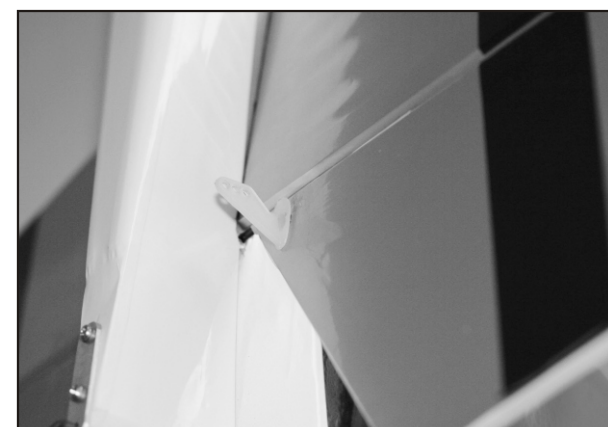
20. Same way as the installation of aileron control horn. Install the elevator control horn in place as shown.
