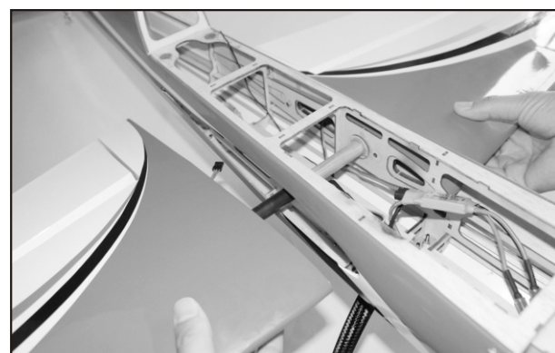
28. Trial fit and main wing in place, then install wing joiner. Locate the Nylon retaining screw then screw in the wing in place as photo shown in next step.
