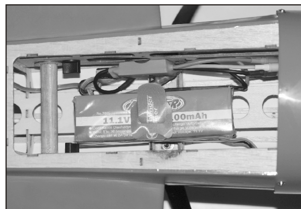
29. Secure the battery with the tie belt as shown in the fuselage.
