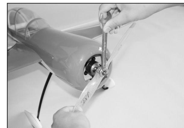
37. Secure the propeller properly with prop nut. Now you finish the assembly please well adjust the control throw and CG before you go to fly.
