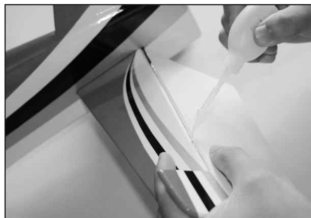
13. Apply epoxy in the elevator torque rod holes then attach the elevator onto the stab. Make sure it moves free after cured.
