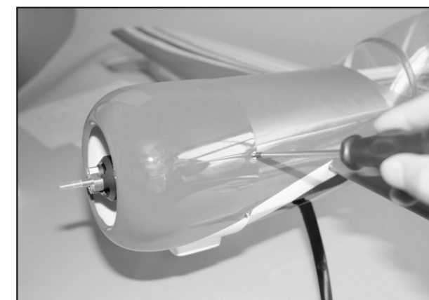
36. Trail fit the cowling in place, make sure the prop adaptor is out of the cowling. Secure the cowling with four 2.3x8mm wood screws.
