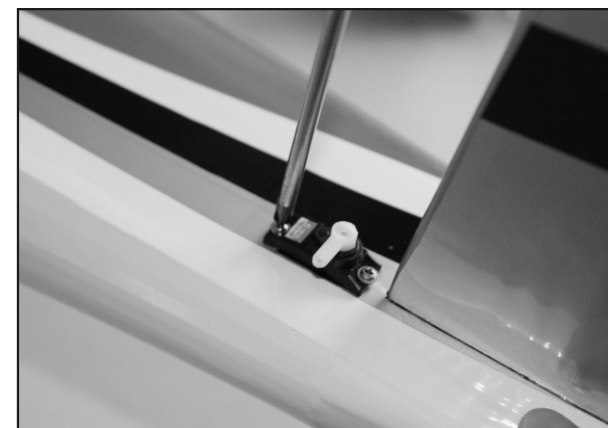
19. Install the elevator servo as shown at the left side of fuselage. Remember connect the extension wire at least 12".
