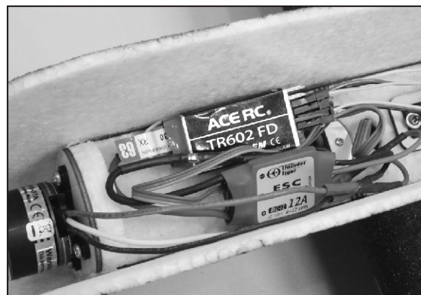
17. Connect the receiver and controller properly, secure these electric devices with the furnished wide Velcro.
