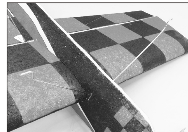
22. Trial fit the landing gear wire and mount first, CA the wire and landing gear mount in place when satisfied. Note two landing gear wires are angled properly.
