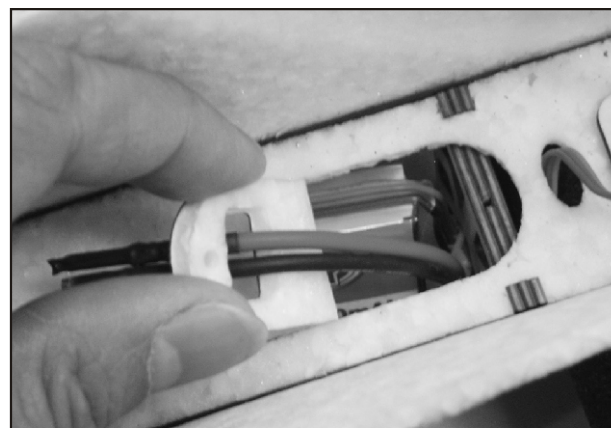
16. Open the hatch and place the Lipo battery in the compartment. Secure the battery in place with the 2.3x12mm wood screw.
