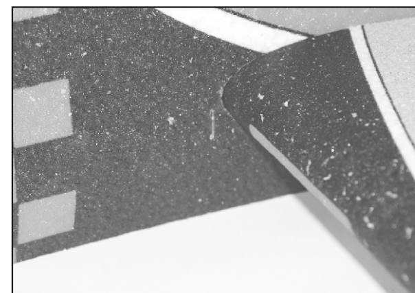
21. Locate the landing gear mounting slot where near the leading edge of main wing as shown.
