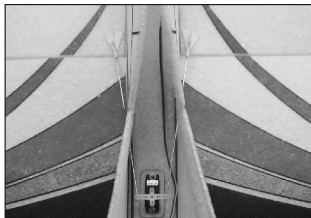
13. Secure the aileron servo and attach the aileron pushrods as shown.
