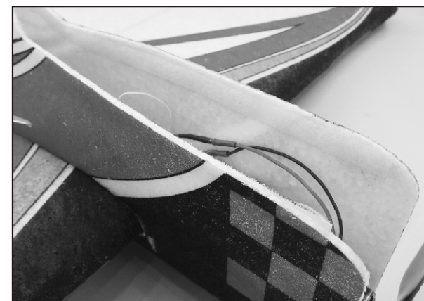
19. Apply the furnished glue on fuselage opening and Velcro, wait for 10 minutes before gluing them together. Hint: It is very important to wait for couple minutes before gluing together. You may blow the glue area and it will be cured faster. Do not separate the Velcro. Carefully attach the Velcro to the fuselage opening on one side first then apply the other side of fuselage to the Velcro.
