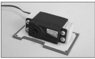
10. If you would use Flap function then proceed the following steps. If not then skip to step 24. Do the same procedure for Flap Servo Case. (Left Flap Servo Case shown) and thread the wire through the wing panel and tape the wire end on wing root.
