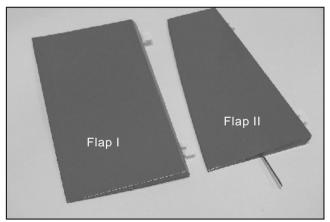
18. Insert guide tube in Flap I and light apply CA glue. Glue threaded end of joiner wire in Flap II, also apply a drop of CA glue. Cut two hinge slots and glue CA hinges in place.
