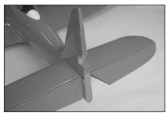
61. Glue Vertical Fin Bracket in place and make sure the upper one and lower one are in line. Apply epoxy at torque rod hole next install the elevator in place. CAall hinges and make sure elevator is firmly secured. 使用環氧樹酯將後緣木粘合到垂直翼上。將升降舵固定到 水平翼,使用瞬間膠水固定活頁確定其牢固不脱落。
