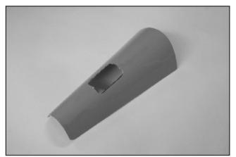
74. Locate the bottom tail cover, make the opening according to the tail gear. 尾蓋須依據尾輪組尺寸及位置開孔。
