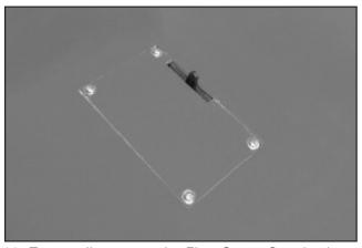
11. Temporally secure the Flap Servo Casein place with 2.3x12mm Washer Wood Screws.
