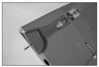
28. Insert the pushrod from wingroot then connectto retract. Note: The ballend with "Tiger" side should face upside of wing. 將推桿自翼根插入自輪座探出 並與脚架連接頭連接。注 意連接頭上"Tiger"字樣朝向上翼面。
