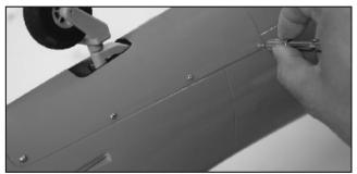
75. Trim the tail cover and fit in place. Drill eight 1.5mm holes then glue doublers at the hole area. It might be needed to sand the doubler to adapt to the curve surface. Drill the holes again on doublers then secure the bottom tail cover with 2x8mm washer wood screws. 將尾輪組蓋子與機身配合定位、 使用紙膠帶暫時固定後 開8個 1.5mm 的孔位。蓋子裡側可能需要使用銼刀或砂紙
