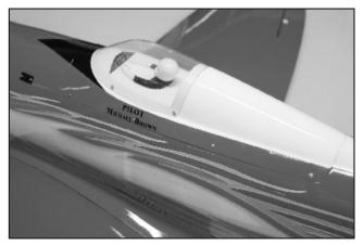
94. Trial fit the upper Cockpit on fuselage, drill eight 1/16" (1.5mm) holes and glue small plywood doublers inside the fuselage at the holes area. Drill the doublers again and secure the cockpit in place with 2x8mm washer wood screws.
