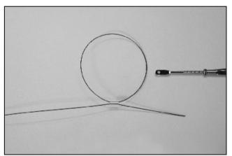
63.Locate the straight threaded end, brass tube, M2 nuts, clevises and wire. Cut wire in length 90mm. First thread the M2 nut and clevis then secure the M2 nut on clevis. Then route the wire through the tube and make it a circle. 组装接桿、連桿頭及 M2螺帽。剪鋼絲约90cm。鋼絲繩先 穿過銅管接著再往返穿過一次(如圖示)。
