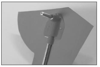
34. Secure the lower retainer on wheel door with two 2x5mm wood screws.
