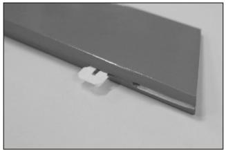
50.Cut away the covering of leading edge at the root of elevator where the torque rod is going to be installed. CA three hinges in elevator at this time. 切開根部隱藏的升降舵控制桿固定槽,以及安装活页片。
