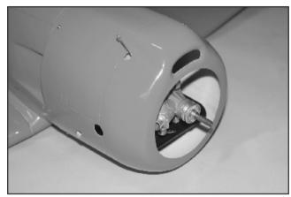
88. Drill needle valve extension wire exit hole. When satisfied, secure the cowling in place with 2.3x12mm Washer Wood Screws.Suggest to install Precision Fueler (TTR1115) for easy fueling.
