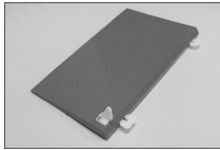
19. Secure control horn on Flap I with 2x15mm machine screw. Note the control horn should away from the edge at least 8mm. The 8mm is to clear the rib located at the center of both flaps.
