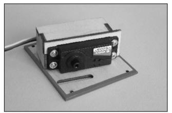
5. Locate the left wing servo case /hatch cover; secure the aileron servo as shown.
