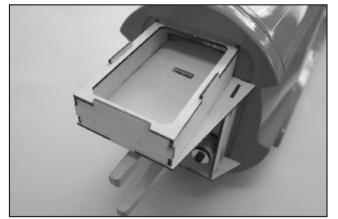
46. Trial fit the battery box, then epoxy the battery box and bottom reinforced ply in place. When cured, lightly apply epoxy on all firewalls area as well as the battery box so the plywood could be fuel-proof. Just mix the epoxy with nomore that 50% mix of alcoholthen brush on firewall.
