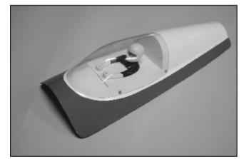
91. Apply instrument panel in the cockpit. Next trim the canopy and trial fit the canopy on the cockpit. Glue the plywood doublers and drill four 1/16" (1.5mm) holes. Secure the canopy with four 2x5mm washer wood screws. Pilot shown is not included.
