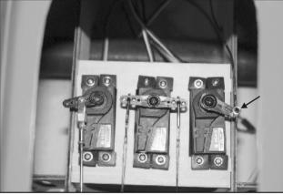
80. Install the EZ connector on the throttle servo horn with M2 washer and M2 nut. Afterwards, thread the throttle pushrod through the EZ connect and secure the servo horn on the servo. Adjust the servo with the radio on, once satisfied with the result, proceed to secure the throttle pushrod with a 3x3mm set screw.
