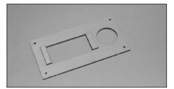
81. Locate the retract servo tray, glue the doubler as shown. Then, install the retract servo on the servo tray. 黏接補強片於收腳伺服機座上。固定收腳伺服機於伺服 機座上。
