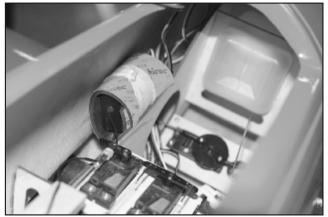
85. Connect all servo wires to the receiver; wrap the receiver with foam to fully protect the receiver. Insert receiver between frame and fiberglass wall in fuselage. 連接伺服機線至接收機。將接收機裹以泡棉保護。將接 收機置於機身與側板之間。
