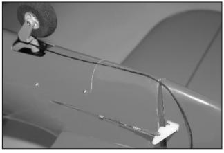
86. Route the antenna along the fuse lage and exit at the tail gear opening. Tape the wire in place as shown. 將天線穿過機身並穿出機尾蓋並以膠帶固並於機身上。
