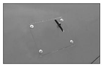
8. Link aileron servos wires to CH1 on receiver. Make sure the direction is correct. Set the servo horn in the neutral then secure the servo horn screw next secure the servo case in place with four 2.3x12mm washer wood screws.
