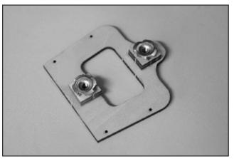
68.Locate the tail gear mount, doublers then glue them together then press the Blind Nut in the hole. It will be easier to use hammer or mice. 將補強合板粘上然後按上盲孔螺帽,最後使用鉗子或是
