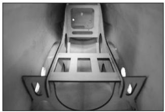
38. The side frame is either marked Lor R.Make sure L is at left side and R is at right side. Always trial fit all wood parts before you glue it. Suggest to glue the one side frame in place first, next the other side frame with servo tray at the same time. Fuel tank retainer and retract servo mount strips at the last.
