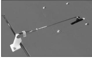
9.Please note that the aileron is thick; carefully drill the (5/64")2mm holes and make sure the back plate is flush with the hingeline at the other side of aileron. Secure the control hornin place with 2x22 machine screws. Trim away the excess screw from the backplate. Install the pushrod with metal clevis, M2 nut and thread on a piece of silicone tube asshown.
