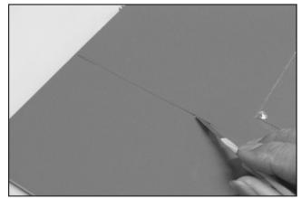
12. Carefully cut away covering. The knife may lean against the flap then carefully cut along with the flap leading edge.
