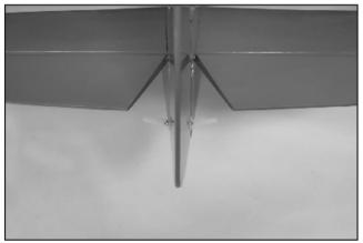
62.CA the Rudder on Vertical Fin with three CAhinges. Next install the control horns on the rudder with two 2x30mm machine screws and M2 nuts. 方向舵以同樣的方式固定在垂直翼上面。 其次安裝舵角
