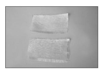
54.Locate the fiber cloth then cut into two pieces at about 100 x 80mm (4 " x 3"). 使用套件內附的纖維布分割成2块为100X80mm。
