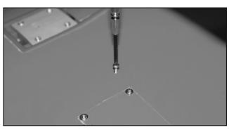
41. Locate the hole that is located at the bottom wing between retract the flap servo hatch. Drill a 5/64" (2mm) hole through the fiberglass tube of the main wing halves, and make sure they are firmly close to the fuselage then secure 3x20mm wood screws. Main wing is removable for convenient in transportation. For best performance, epoxy two wing halves is strongly recommended. 於下翼面找出主翼固定孔,確定主翼與機身密合鑽以2mm 孔再以 3x20mm木螺絲固定。建議以環氧樹酯膠合主翼與 機身,减少主翼振动避免影响飞形性能。
