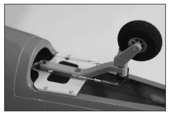
72. Do the same procedure of the pull-pull wire on tail gear. 尾輪方向控制裝法如同方向舵。
