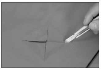
Locate the aileron servo well then use a hobby knife to cut an "X".
