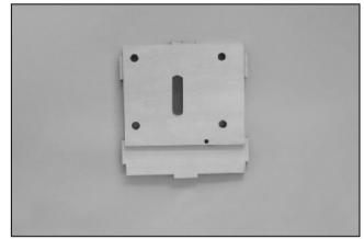
42.Sandwich the three firewalls together; note the cross laser cutmark should be on the top and smallest one at the bottom.
