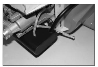
79.Install T tube fitting and fuel tube plug as shown, this will help you to know fuel is full when pumping. 建議安裝三通於油箱回壓與消音器之間以檢視加油滿油 情形。
