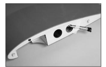
23. Epoxy the dowels at wing root in place as shown. 膠合固定销於主翼上。
