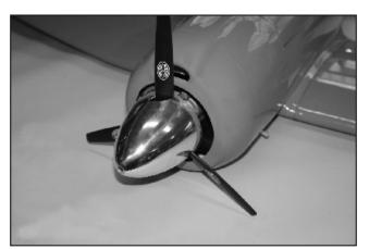
89. Install the propeller and furnished spinner. What we used here is Master Airscrew 13x8. 安裝機頭罩及螺旋槳, 建議使用Master Airscrew13x8 獎搭配TT PR0-91。
