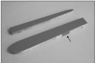
60. Trail fit the Vertical Fin Bracket in the Vertical Fin, you may need to sand to fit in place. When satisfied, use furnished covering and iron on the covering as shown. 圖示為垂直尾翼的後緣,裝在垂直翼上可能須適度使用砂 紙修整。請注意包覆紙之包覆保留侧面如图所示。
