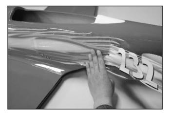
92.Refer to the box label then apply all decals. Suggest to join the fire decals together before applying on fuselage. 參考飛機彩盒圖片黏貼貼紙,建議將火焰貼紙先結合再貼
