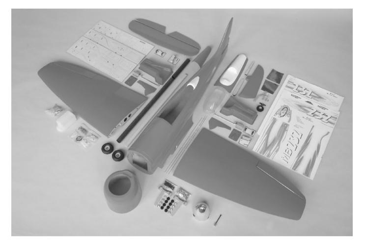
Kit Contents: FRP Fuselage(1) FRP Cockpit(1) FRP Tail Cover (1) FRP Cowling (1) FRP Wing Joiner Tube (L/1) FRP Tube (S/1) Left Wing (1) Right Wing (1) Right Wing (1) Rudder (1) Horizontal Tail (1) Elevator (L/1, R/1) Aileron Servo Case (L/1, R/1) Flap Servo Case (L/1, R/1) Plywood Parts(A) Plywood Parts(B) Plywood Parts(C) VT Lower Trailing Edge (1) VT Upper Trailing Edge (1) Doubler(28) Dowel (4) Covering (1) Fiber Cloth (1)
