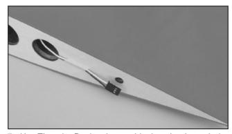
7. Use Throttle Pushrod to guide the wire through the wing panels. Fix the wire with mask tape to prevent from falling back into wing pannel.
