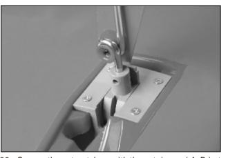
33. Secure the retract door with the retainers (A,B) at the strut coil with 2.6x5 mm wood screw. 拉起起落架裝置輪艙蓋,並以2.6x5mm木螺絲固定輪艙蓋 固定件A與B。
