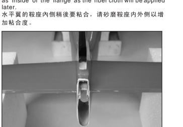
53. Insert and center the tail in place. Use books or boxes to support tail ends make sure it is level to the main wing. You may need to file the flange to get a good fit. Use furnished rubber bands to reduce the gap and fix the tail in place. Apply thick CA or epoxy when satisfied.
