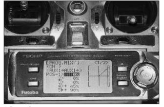
1.Reset first. 2.Flap ATV 140% 140% 3.AUX1 ATV 140% 140% 4. Airbrake on Flap 100% 5.PMIX7 AUX1-AUX1 Position 1:0% Position 2:0% Position 3:0% Position 4:45% Position 5:90% 6. Trim the two flaps at same throws by adjusting the trim knob and pushrod if necessary.
