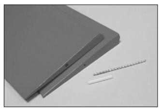
16. Locate the joiner wire and guide tube. Make mark at the center of the joiner side of the Flap I and Flap II. 設置連動钢丝以及導管。在內、外側襟翼的中間做記號。
