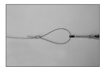
64. Next thread the wire through the clevis linkage then tread to the tube again. 穿過連接桿组返穿回銅管(如圖示)。
