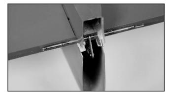
58. Apply a small tube onto the clevis then connect the elevator pushrod to the elevator torque rod. A flat head screwdriver will help snapping the clevises onto the torque rod link. Trim the elevator center notch for enough throws (down) as page 24 shown. 將推桿連桿頭連接至升降舵控制桿上面的舵片。使用銼
