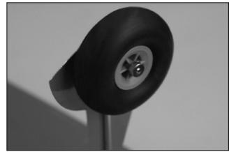
35.Install the wheel and secure collar with 3x3mm set screw. Make sure wheel rotates freely. 安裝輪胎并用輪擋及3X3mm的無頭内六角螺絲固定。
