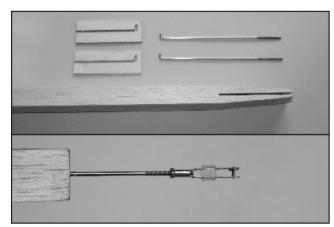
57.Locate the elevator pushrod parts asshown, epoxy the plywood inside the wood rod at two ends with wires. Thread the M2 nuts and clevises and make surethe whole elevator pushrod has no free play. Note the orientation of the pushrod andclevis.
