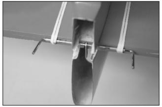
56.Lubricant oil to the hinges of elevator torque rod. You may spray WD-40 on the hobby knife then use the knife tip to contact the torque shaft and the oil will go into the hinge. Epoxy the elevator joiner in place.
