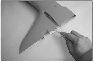
47.Remove the balsa insert from the vertical fin. Then use flat file to file thein side of the tail to get a smooth surface.
