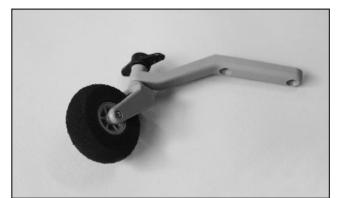
70. Locate the tail gear bag, and assemble the tail gear as shown. Note the orientation of steering arm, trim the outer hole away as it is too long to install in the tail. Secure steering arm in place with 3x5mm set screw. 打開尾輪組零件包開始裝配尾輪組。注意控制臂的方向, 控制臂最外面的孔位必須切除、否則會發生干涉的狀況。 控制臂使用3x5mm螺絲固定。
