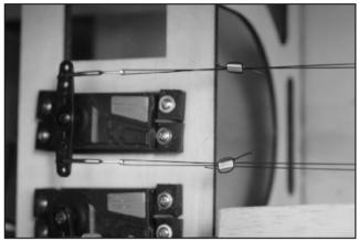
73. Adjust the threaded end at the servo end to get better tension of the four wires and make sure both rudder and tail gear are in line with each other. Crimp the tubes when satisfied.
