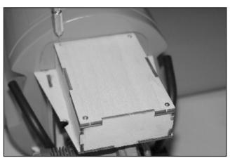
84. Secure battery box cover with four 2x8mm washer wood screws. 以2x8mm 墊片木螺絲固定電池盒蓋。
