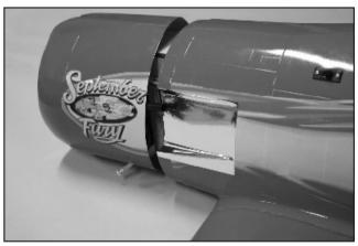
95. You may need to remove the cowling and apply silver decal as shown. 暫時卸下引擎罩並貼以銀色貼紙於排氣處。
