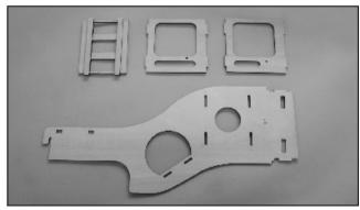
37.Locate servo trays and servo tray doubler then glue the doubler in place. There are two fuel tank frames. Make sure the shorter slot is in the front and longer slot is in the rear.
