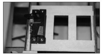
59.Install elevator servo, note the servo horn orientation. Then adjust the clevises to make sure elevators are level when servo is in neutral position. When satisfied, remove the elevator pushrod temporarily and secure M2 nuts and clevises firmly.
