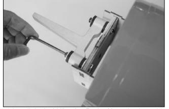
45.Install the Anti-Vibration Engine Mount in place with 5x40mm Socket Cap Screw and Blind Nut. You just screw in the cap screw then the blind nut will punch into the firewall.
