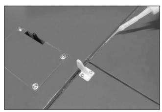
21. Join two flaps then insert them to the wing in place. Make sure there is no contact with each other then apply CA at the hinge area. Move the flap again and make sure it works smoothly.
