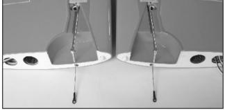
29. You may need to trim the wires of retract so the wheel axle is lever to the wing root. Secure the retract in place with four 3x15mm Sink Head Screws. Flats should be ground on the landing gear legs for the setscrew to prevent the wheel axle from rotating under load. 先切除多餘的起落架钢丝, 長度与翼根切齊, 然後使用 3x15mm 的沉頭木螺絲固定起落架。輪軸與起落架固定的地方必須磨一個平槽以有效固定輪軸。
