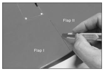
13. Next cut away the covering between Flap I and Flap II. 開縫式襟翼分內外側兩片、请小心切開。
