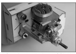
77. Remove the engine and engine mount. Drill the 3.4mm holes based on those marks then tap the hole with M4x0.7 thread tap. Connect throttle pushrod then secure the engine with M4x20mm socket cap screws. Make a Z bent on throttle pushrod as indicated.
