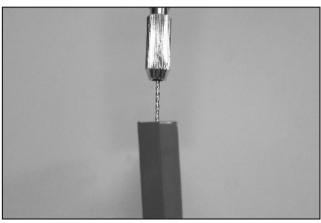
17. Carefully drilling the joiner side at mark. Note that it is angle at the joiner side please drill the hole perpendicular to the surface. Drill 2.5mm hole on Flap I and 2mm hole on Flap II.
