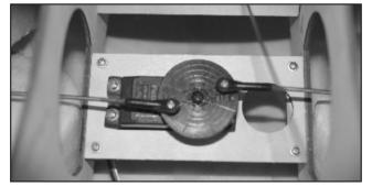
82. Secure the whole assembly in place with four 2.3x12mm washer wood screws. Next secure two Steel Balls on the servo horn with 2x8mm machine screw and M2 nuts. The distance between two balls is 24mm. Fine adjust the retract pushrod, and make sure the ball link with "Tiger" is facing up. Switch on the retract gear to make sure the retract gear works smoothly.
