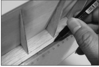
20. Leave 0.5mm clearance between ribs and flap then draw the hinge line. Next cut hinge slots to accommodate the hinges on flaps.
