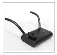
Muffler (P/N TTR9791) Most Pitts style mufflers will fit this Sept. Fury. However, we recommend the use of Thunder Tiger custom - made Sept. Fury muffler with two exhaust pipes that divert the smoke in to the two concavities of the fuselage to obtain a more scale- like apperance. This muffler fits TT and OS. 60~.90engines.
