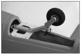
71. Secure the tail gear assembly on the tail gear mount with 4x20mm sink machine screws. 尾輪組使用4x20mm平頭螺絲固定在尾輪座上。
