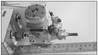
76. Place the Engine (Thunder Tiger PRO-91 Shown) in the Engine Mount then proceed to make mounthole marks on the engine mount where drive washer is 5 3/4" (147mm) to the firewall.
