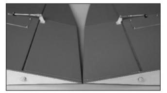
22. Repeat the same procedure on the right wing. Link two aileron servo wires with Y cord and plug to CH1 on receiver. Plug the left flap to Ch6 and right flap to Ch7. Refer to your radio manual and set up Flap.
