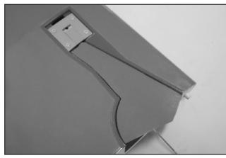
31. Trim the retract door to fit the retract well. 修整輪艙蓋并確認与輪艙搭配完美。
