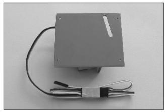
6. Connect an extension wire for Aileron servo, heatshrink or tape the connectors to prevent from loosening.
