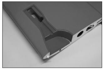
25. CA the retract well in place, trim the excess plastic so it is level with the wing root. 以瞬間接著剤將輪架真空罩固定於主翼上,並與翼根修齊。
