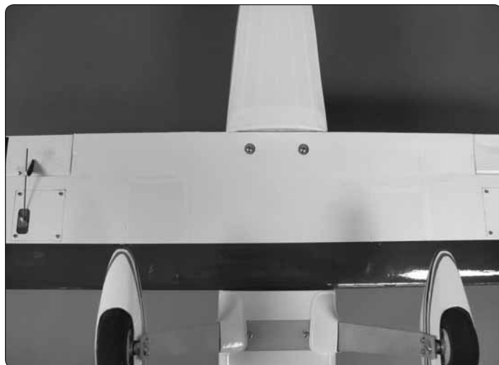
❑ 5. Bolt the bottom wing to the fuselage with two 4-40 x 1" wing bolts and #4 flat washers.
