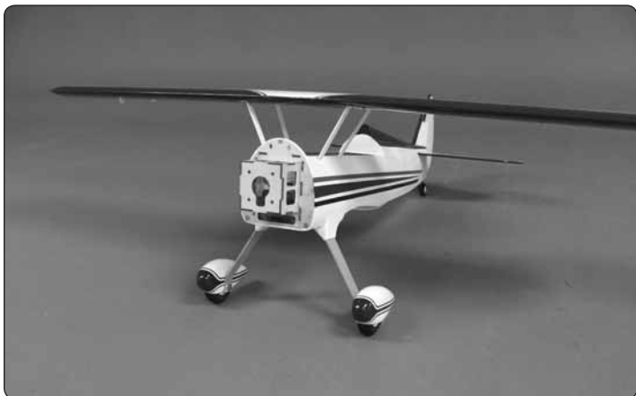
❑ 4. Attach the top wing to the cabanes with four 2-56 x 3/8" [9.5mm] machine screws. Be sure to use a couple of drops of thread locker on each of the screws before installing them.
