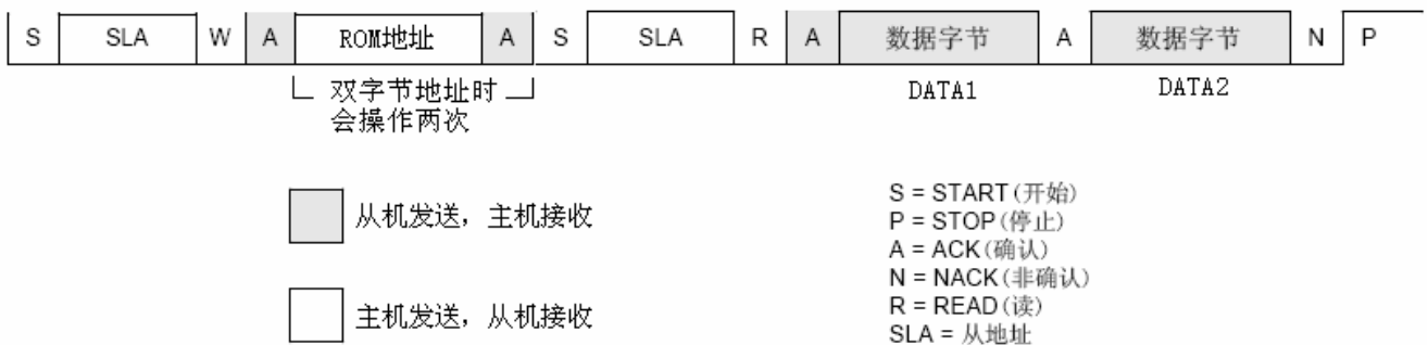
USB-I2C Adapter I2C Read Timing
