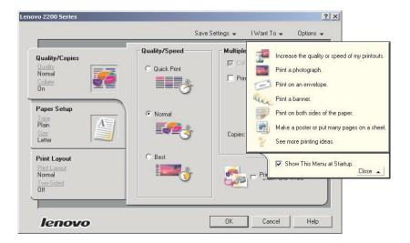
You can change your printer settings in the printer driver. To print a typical document on plain paper, you do not need to change your printer settings. When you install the printer software, the Page Setup dialog box and the Print dialog box are set to these default settings:
