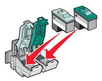
**Note:** To extend the life of your color cartridge and improve printing speed, install a black cartridge along with the color cartridge.
