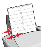
**Note:** If you are using letter size sheets of labels, adjusting the paper guide may not be necessary.
