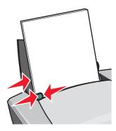
Note: If you are using letter size paper, adjusting the paper guide may not be necessary.
