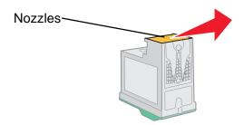
**d** Using another clean section of the cloth, gently hold the cloth against the contacts for about three seconds, and then wipe in the direction shown.
