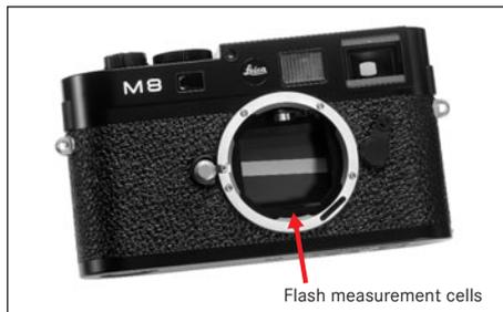
The LEICA M8.2 determines the necessary flash power by firing one or more ranging flashes, fractions of a second before taking the actual picture. Immediately after this, at the start of exposure, the main flash is fired.
