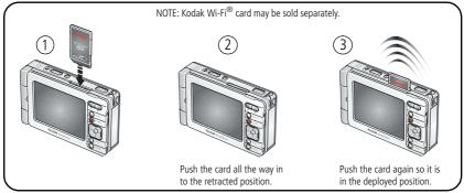
When possible, keep the Wi-Fi card in the retracted (2) position for safe-keeping and to conserve battery life. To connect to an available Wi-Fi wireless network, push the card in so that it springs back up to the deployed (3) position (see page 45).
