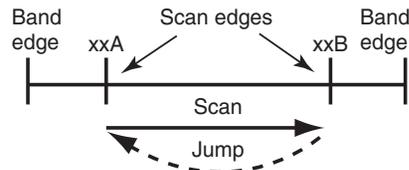
Repeatedly scans between two user-programmed frequencies. Used to check for frequencies within a specified range, such as repeater output frequencies, etc.
