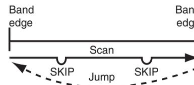
Skips unwanted frequencies or channels that inconveniently stop scanning. This function can be turned ON or OFF by pushing **[FUNC] + [SKIP](V/M)** in either the VFO or the memory mode.
