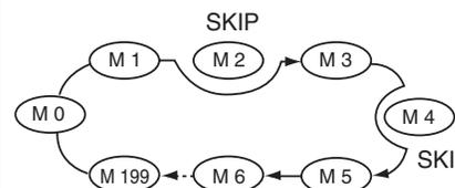
Repeatedly scans memory channels, except those set as skip channels. Skip channels can be turned ON or OFF by pushing **[FUNC] + [SKIP](V/M)** in the memory mode.
