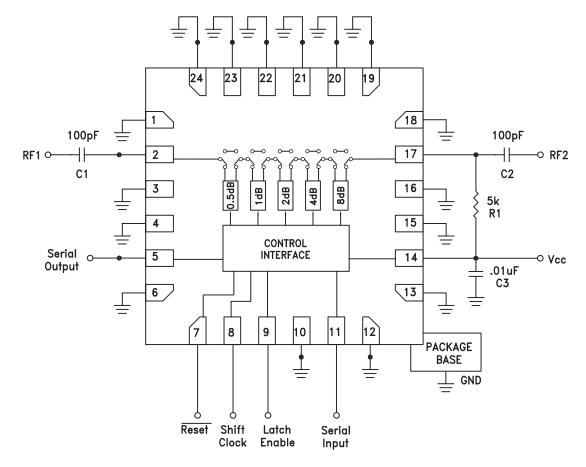
DC blocking capacitors C1 & C2 are required on RF1 & RF2. Choose C1 =  $C2 = 100 \sim 300$  pF to allow lowest customer specific frequency to pass with minimal loss. R1 = 5k Ohm is required to supply voltage to the circuit through either PIN 2 or PIN 17.
