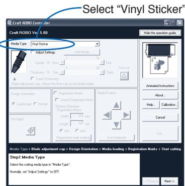
Select "Vinyl Sticker" in the Media Type box. Click the [Next] button to proceed to the "Blade cap adjustment" step. Install the blue cap displayed on the screen to the blade holder tip.
