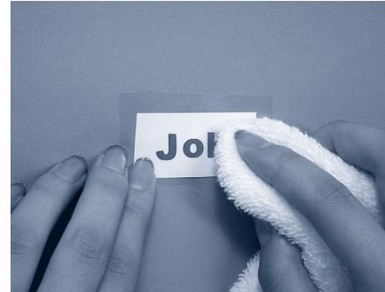
After affixing the application sheet, rub it firmly with a cloth or something similar to transfer the cut characters onto the sheet.
