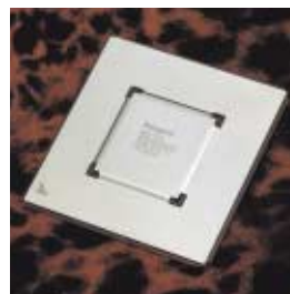
Next-generation digital process ASIC (0.18 \mu m design rule)
