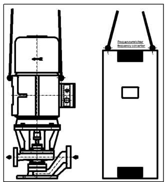
A crane must be used for all pump sets in excess of 25kg (55lb). Fully trained personnel must carry out lifting, in accordance with local regulations. The driver and pump weights are recorded on their respective nameplates.
