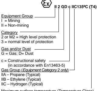
Maximum surface temperature (Temperature Class) (see section 1.6.4.3)
