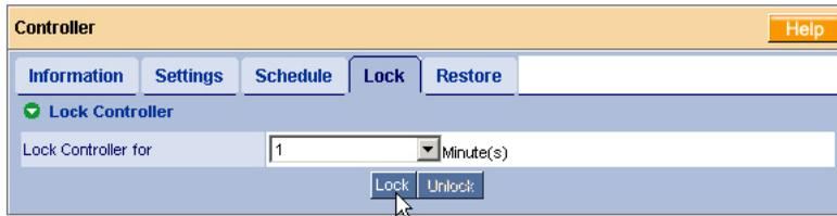
The Lock tab displays lock status and enables you to lock or unlock a subsystem controller. The locking mechanism isolates the controller during maintenance operations and other periods when you want to avoid interruption from other users trying to access the logical drives under this controller.
