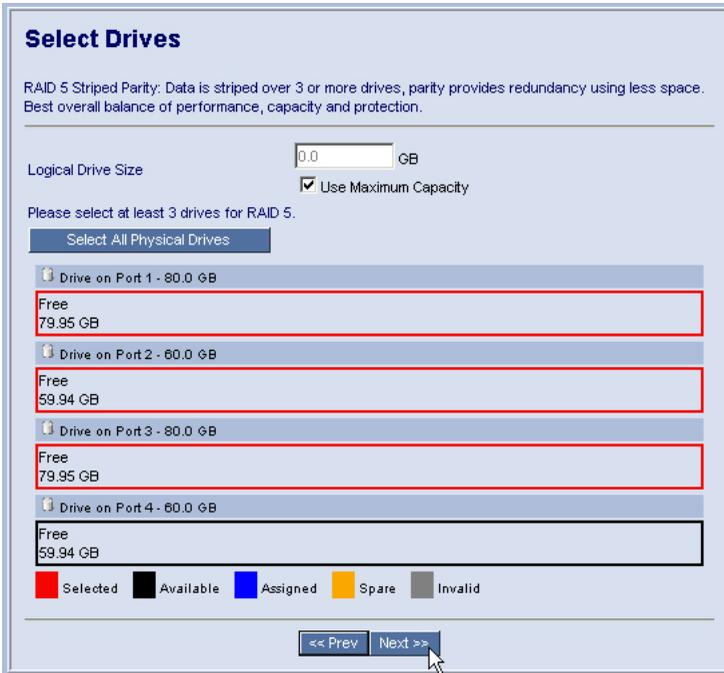
6. If you want to create a logical drive with unused capacity, enter the assigned (used) capacity in the Logical Drive Size field.
