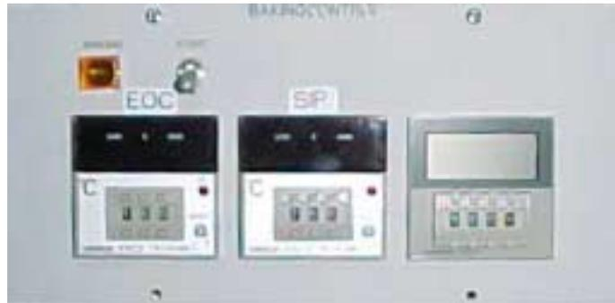
Controls baking operation of the electron gun chamber and ion pumps.
