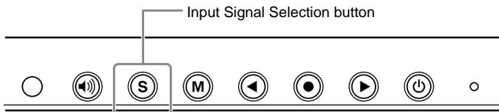
Switch the input signal with **(S)**. Input signal switches each time **(S)** is pressed. When the signal is switched, the active signal type (Analog or Digital) appears at the top right corner of the screen for three seconds.
